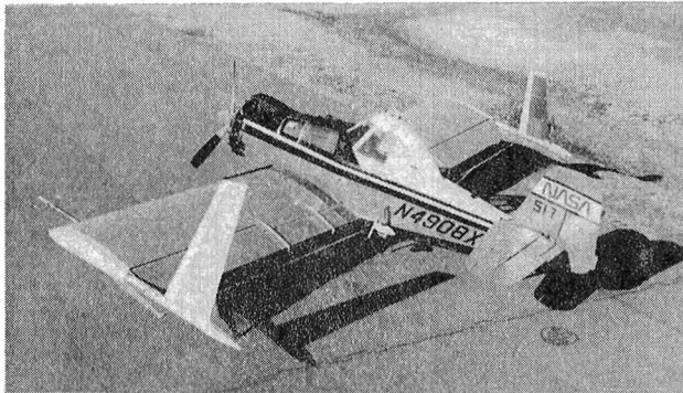
Figure 3. Agricultural airplane with vortex diffusers.
