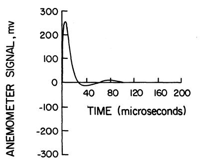
FIGURE 3 - HOT - WIRE ANEMOMETER RESPONSE TO A SQUARE WAVE INPUT.
