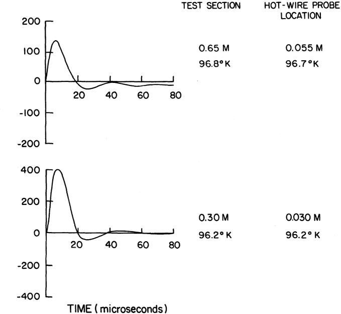
FIGURE 6 - HOT-WIRE ANEMOMETER RESPONSE TO PARTICLE STRIKES AT 5.0 atm FOR TWO VALUES OF CARRIER STREAM VELOCITY.
