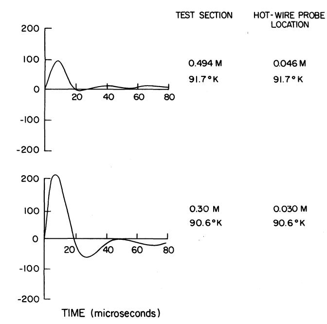
FIGURE 5 - HOT-WIRE ANEMOMETER RESPONSE TO PARTICLE STRIKES AT 3.0 atm FOR TWO VALUES OF CARRIER STREAM VELOCITY.
