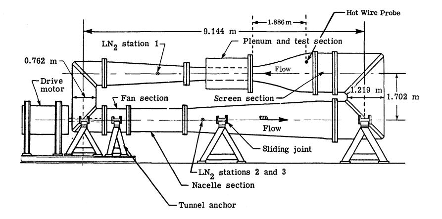
FIGURE I - SCHEMATIC DIAGRAM OF LANGLEY 0.3 METER TRASONIC CRYOGENIC TUNNEL.
