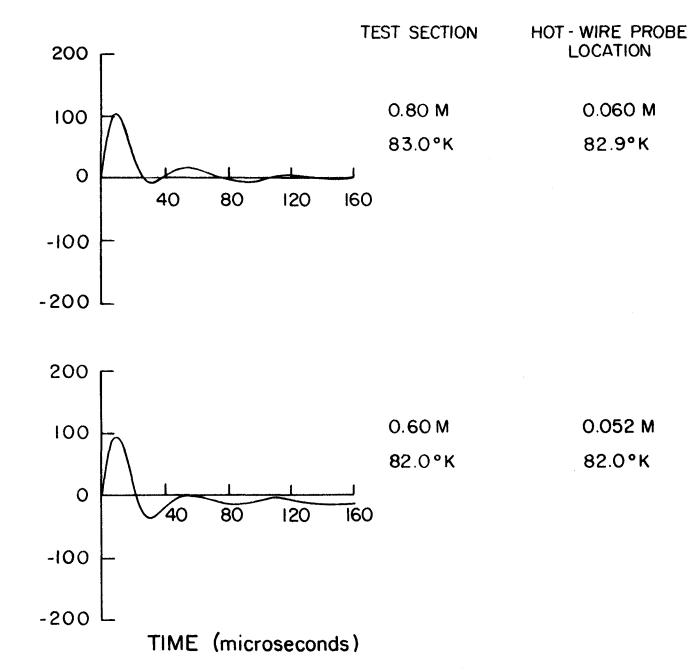
FIGURE 4 - HOT-WIRE ANEMOMETER RESPONSE TO PARTICLE STRIKES AT 1.2 atm FOR TWO VALUES OF CARRIER STREAM VELOCITY.
