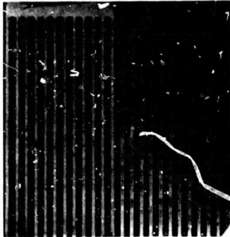
Figure 7. - Silicon surface of a Mg-Ag contacted cell. Ta 2 O 5 coating on left half caused severe pitting during heat treatment.
