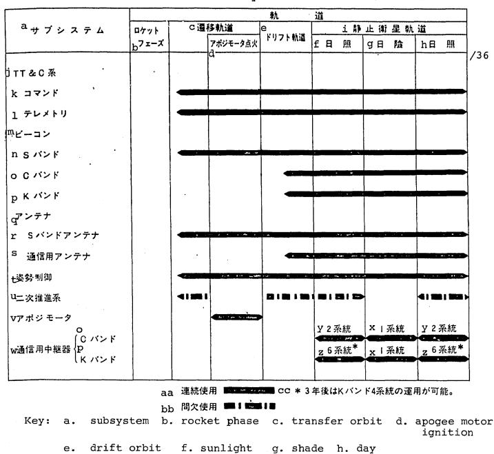
i. geostationary orbit j. TT&C system k. command
