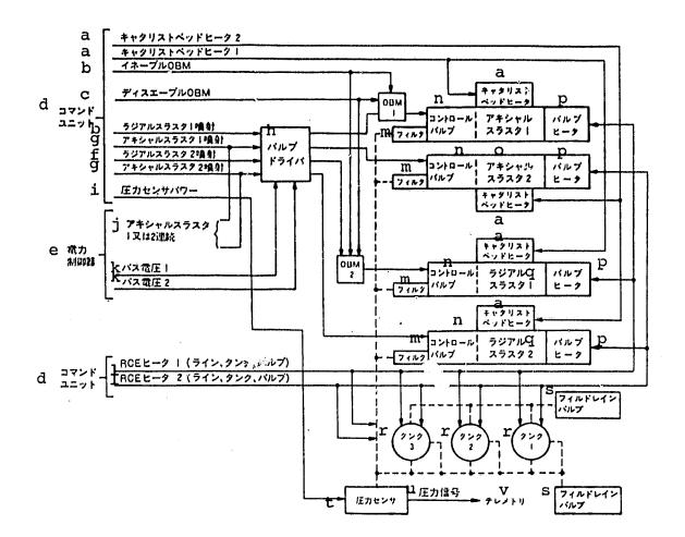
Key: a. catalytic bend heater b. enabling OBM c. disabling OBM đ. command unit electric power control device e. f. radial thruster/jet propulsion g. axial thruster/jet propulsion h. valve driver pressure sensor power i. 1. axial thruster k. bus voltage 1 or 2 connections 1. RCE heater (line, tank, valve) m. filter n. control valve ο. axial thruster valve heater q. radial thruster r. p. tank s. fill drain valve t. pressure sensor u. power signals v. telemetry
