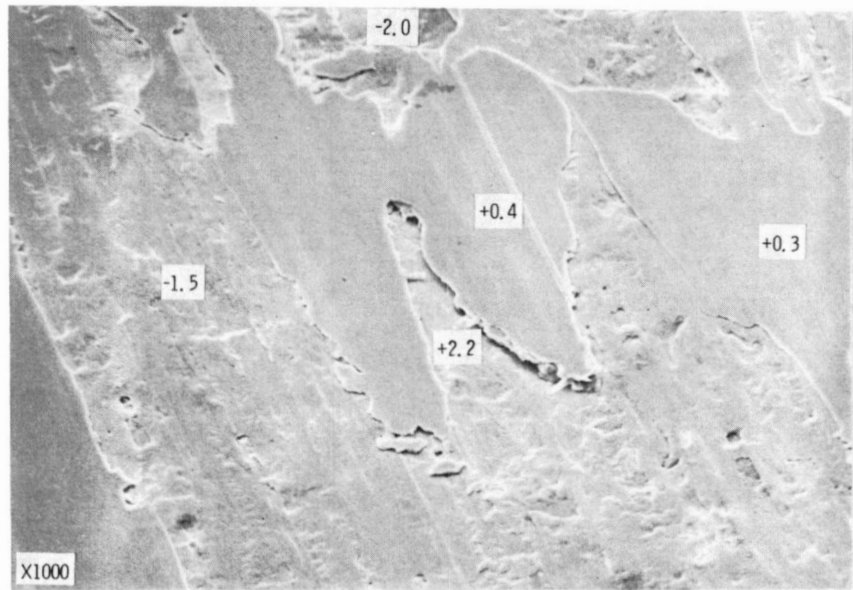
Figure 15. - Plastic deformation on disk surface (VII). 50-pass sliding in 5 \times 10^{-4} -Pa chlorine gas. Figures denote distance (in \mu\text{m} ) from initial height of disk surface.
