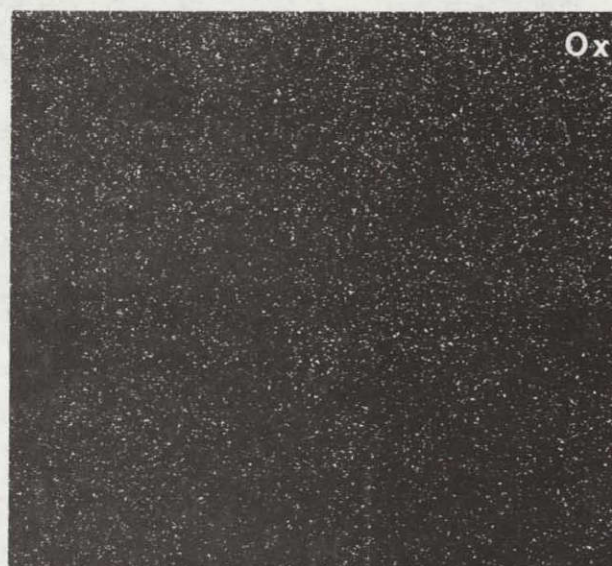
Figure 84 – Elemental Analysis of Impurities in Hot Pressed Mullite
