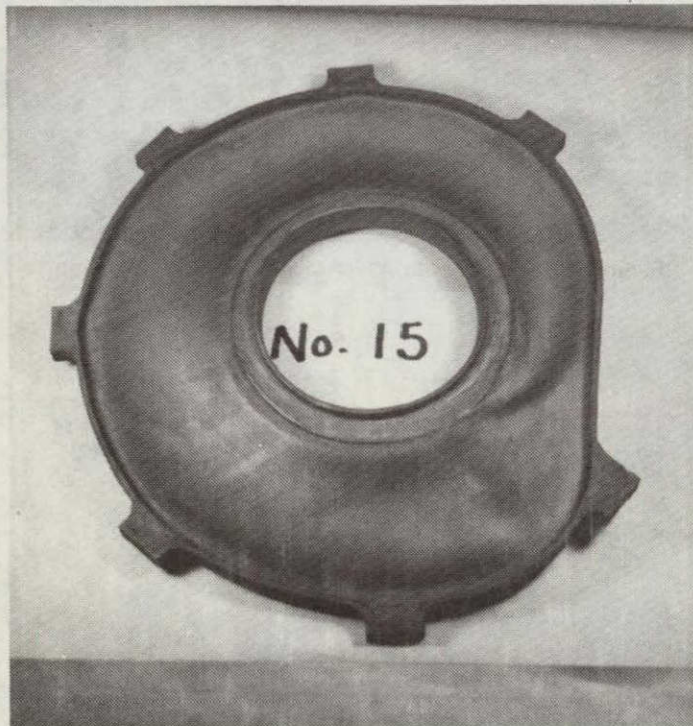
Figure 100 — Sintered Alpha Slip-Cast Gasifier Rotor Scroll Black Plate With Thick Tab and Vane Pocket Regions
