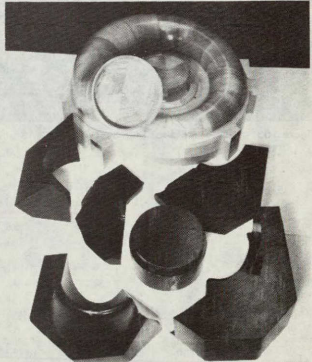
Figure 102 — Epoxy Mold Castings Made from the Original Wood Gasifier Scroll Slip-Casting Pattern
