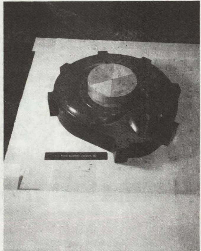
Figure 98 — Epoxy Gasifier Turbine Outer Backplate Pattern for Making Slip-Cast Molds
