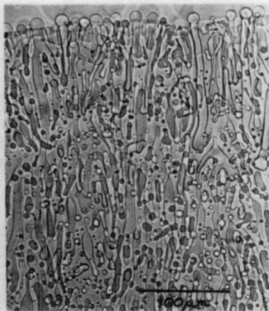
Fig. 2 Succinonitrile ~20 Wt.% Ethanol V = 0.9\mu\text{m s}^{-1} G = 5\text{K mm}^{-1} Transmitted light.
