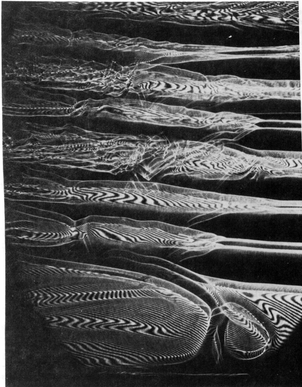
Interference pattern created by horizontal cellular motion resulting from side heating a stable vertical density gradient established by stratified sucrose solutions.
