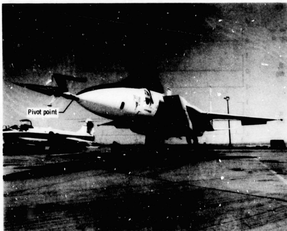
Figure 5. Transition cone mounted in front of test-bed aircraft.
