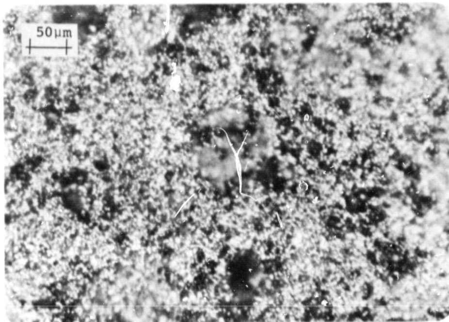
Fig. 4 Optical micrograph of S079A3 print (with eutectic dopant), fired at 500°C (two step) at 200X.
