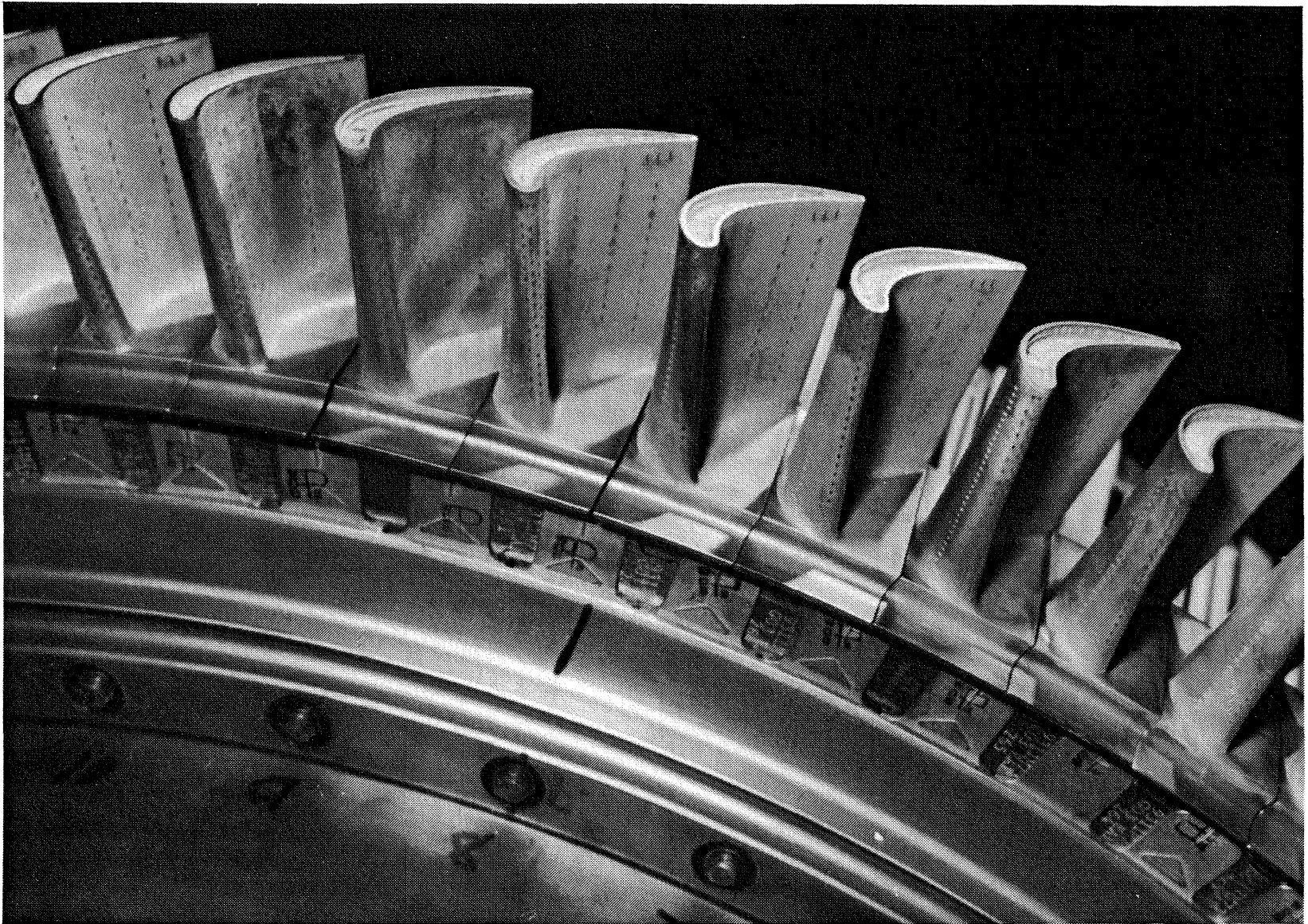
Figure 43. Turbine Blades, with the Advanced Tip System, Assembled into the Rotor. 45.
