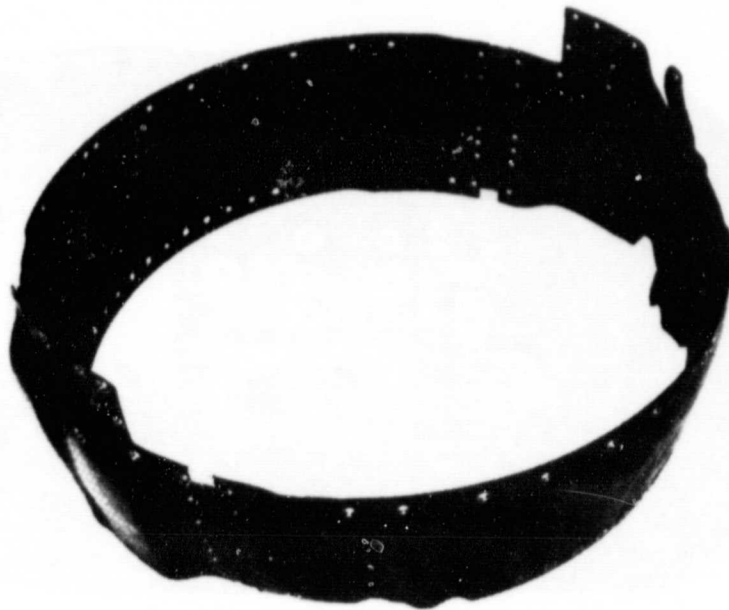
Figure 9. - Graphite fiber/PMR-15 F101 DFE inner duct (Diameter = 102 cm, length = 38 cm, and thickness = 0.15 cm.).
