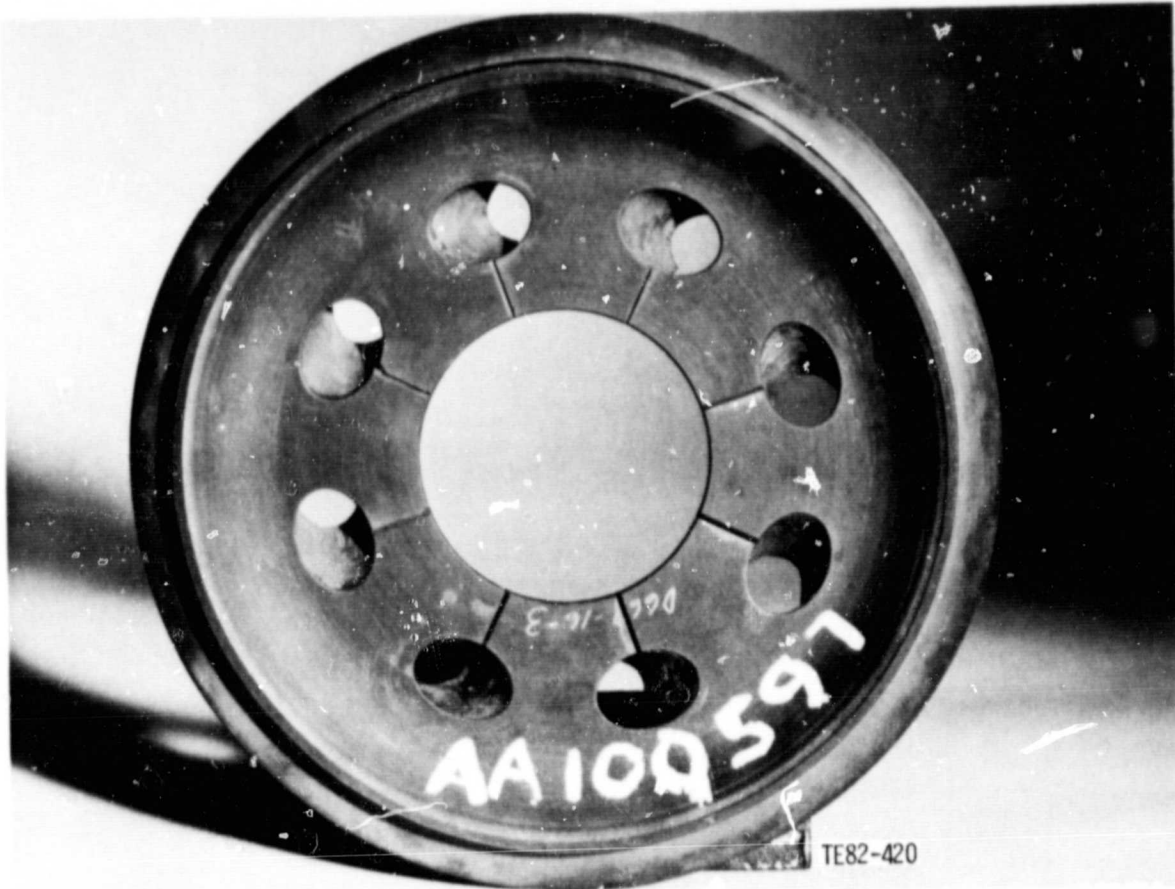
Figure 22. Ceramic combustor swirl plate (dome).
