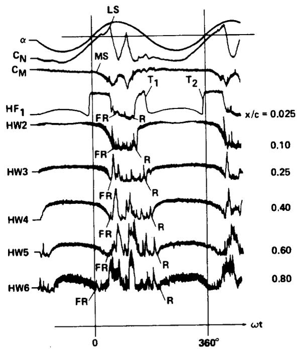
Figure 11.- Response of hot-film skin-friction gage and hot-wire anemometer probes on Vertol VR-7 during oscillation in pitch ( $\alpha = 15^\circ + 10^\circ \sin \omega t$ ,  $k = 0.10$ ,  $M_\infty = 0.185$ ).
