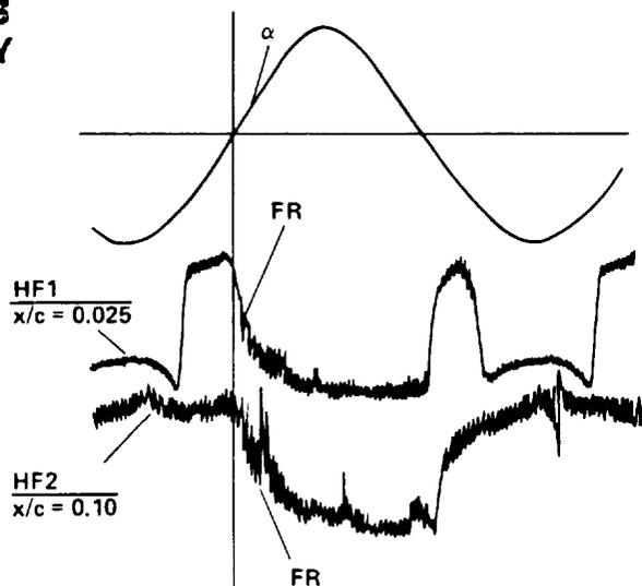
Figure 4.- Response of hot-film skin-friction gages at surface of NACA 0012 airfoil during airfoil oscillation in pitch ( $\alpha = 15^\circ + 10^\circ \sin \omega t$ ,  $k = 0.10$ ,  $M_\infty = 0.295$ ).
