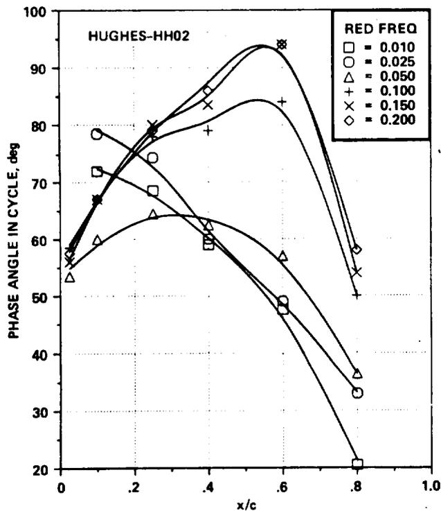
Figure 24.- Phase angle,  $\omega t$ , of flow reversal on Hughes HH-02 airfoil vs chord location for a range of frequencies at  $M_\infty = 0.295$ ,  $\alpha = 10^\circ + 5^\circ \sin \omega t$  - light-stall conditions.
