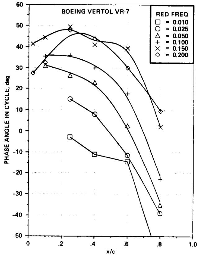
Figure 25.- Phase angle,  $\omega t$ , of flow reversal on Vertol VR-7 airfoil vs chord location for a range of frequencies at  $M_\infty = 0.295$ ,  $\alpha = 15^\circ + 5^\circ \sin \omega t$  - light-stall conditions.
