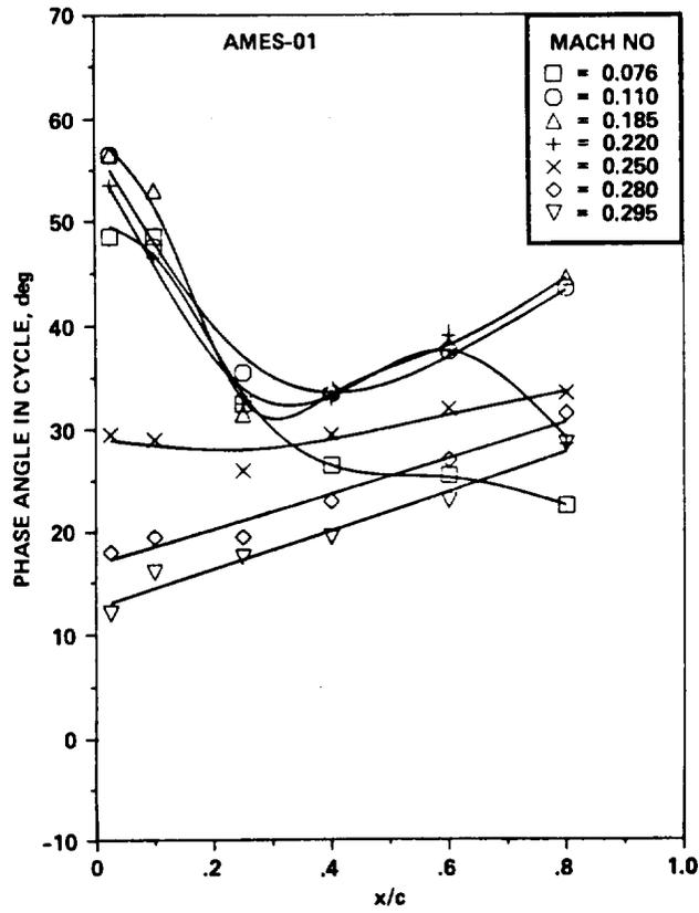
Figure 13.- Phase angle,  $\omega t$ , of flow reversal on Ames A-01 airfoil vs chord location for a range of Mach numbers at  $k = 0.1$ ,  $\alpha = 15^\circ + 10^\circ \sin \omega t$  - Mach number effects.
