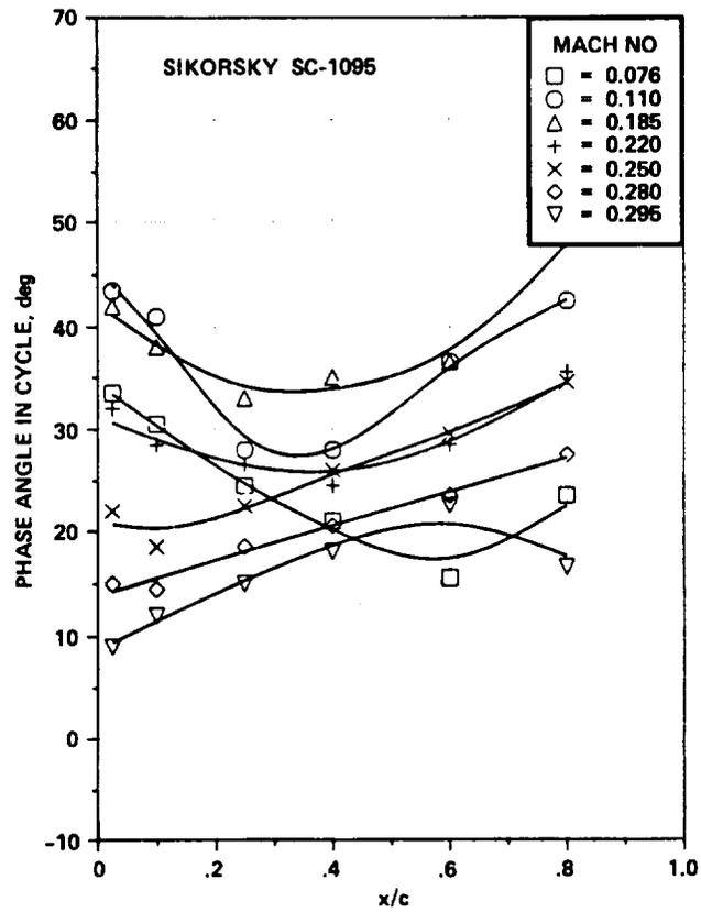
Figure 15.- Phase angle,  $\omega t$ , of flow reversal on Sikorsky SC-1095 airfoil vs chord location for a range of Mach numbers at  $k = 0.1$ ,  $\alpha = 15^\circ + 10^\circ \sin \omega t$  - Mach number effects.
