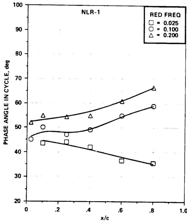
Figure 26.- Phase angle,  $\omega t$ , of flow reversal on NLR-1 airfoil vs chord location for a range of frequencies at  $M_\infty = 0.295$ ,  $\alpha = 10^\circ + 5^\circ \sin \omega t$  - light-stall conditions.
