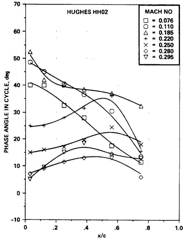
Figure 16.- Phase angle,  $\omega t$ , of flow reversal on Hughes HH-02 airfoil vs chord location for a range of Mach numbers at  $k = 0.1$ ,  $\alpha = 15^\circ + 10^\circ \sin \omega t$  - Mach number effects.
