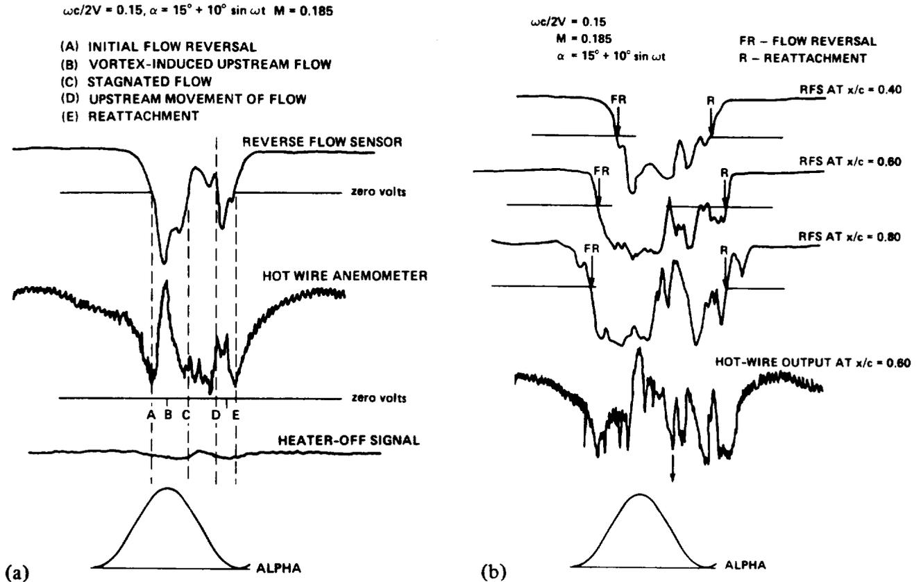
Figure 8.- Results obtained using triple-wire flow-reversal sensor:
