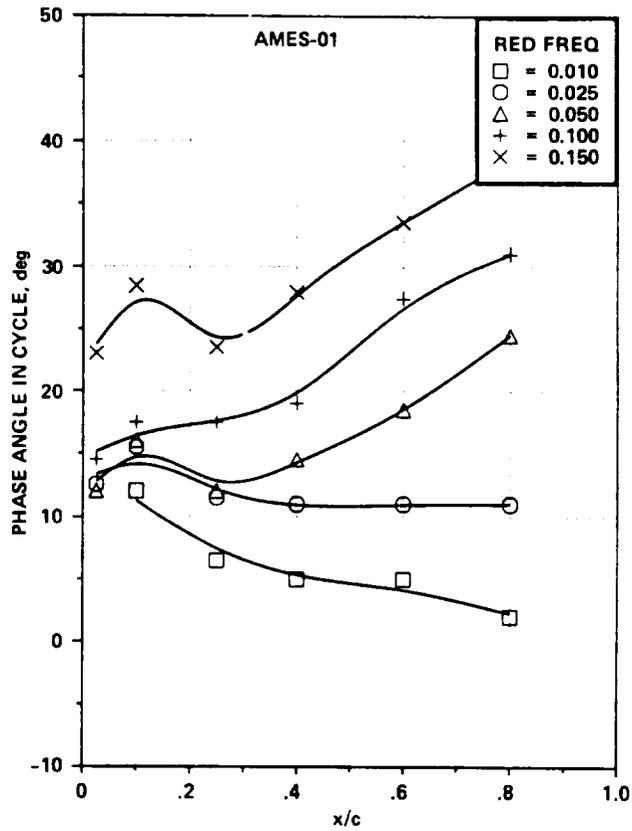
Figure 28.- Phase angle,  $\omega t$ , of flow reversal on Ames A-01 airfoil vs chord for a range of frequencies at  $M_\infty = 0.295$ ,  $\alpha = 15^\circ + 10^\circ \sin \omega t$  - deep-stall conditions.
