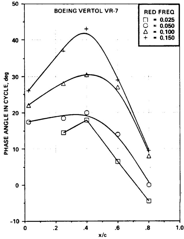
Figure 31.- Phase angle,  $\omega t$ , of flow reversal on Vertol VR-7 airfoil vs chord for a range of frequencies at  $M_\infty = 0.295$ ,  $\alpha = 15^\circ + 10^\circ \sin \omega t$  - deep-stall conditions.
