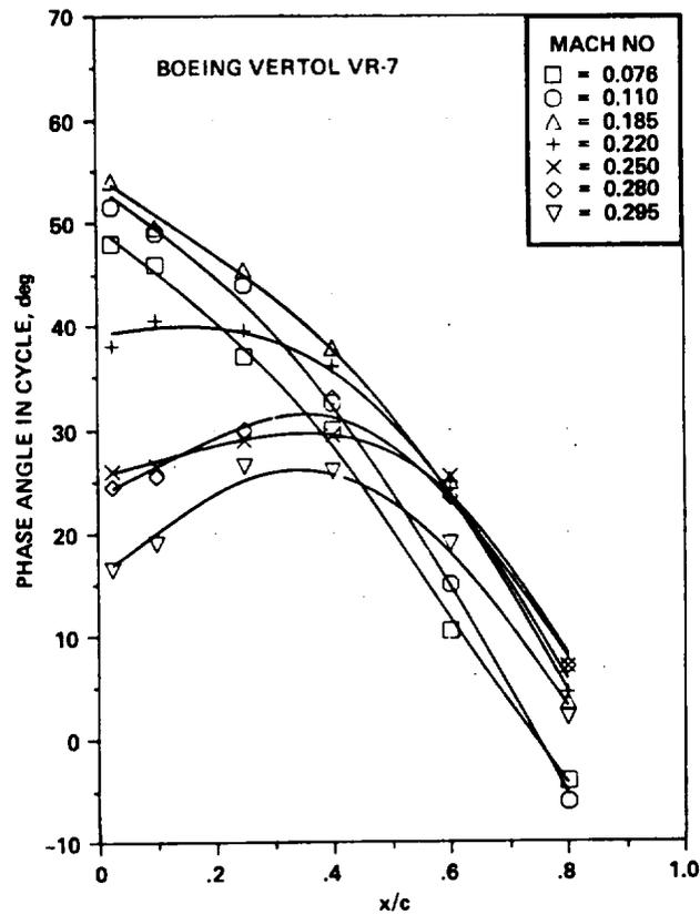
Figure 17.- Phase angle,  $\omega t$ , of flow reversal on Vertol VR-7 airfoil vs chord location for a range of Mach numbers at  $k = 0.1$ ,  $\alpha = 15^\circ + 10^\circ \sin \omega t$  - Mach number effects.
