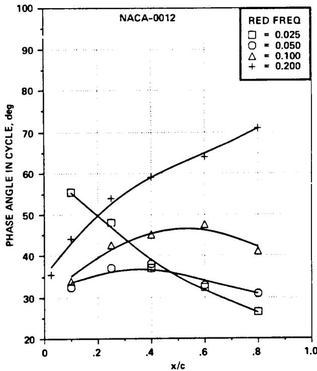
Figure 20.- Phase angle,  $\omega t$ , of flow reversal on NACA 0012 airfoil vs chord location for a range of frequencies at  $M_\infty = 0.295$ ,  $\alpha = 12^\circ + 5^\circ \sin \omega t$  - light-stall conditions.
