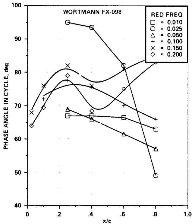
Figure 22.- Phase angle,  $\omega t$ , of flow reversal on Wortmann FX-098 airfoil vs chord location for a range of frequencies at  $M_\infty = 0.295$ ,  $\alpha = 10^\circ + 5^\circ \sin \omega t$  - light-stall conditions.
