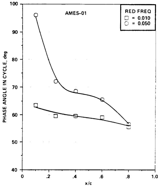
Figure 21.- Phase angle,  $\omega t$ , of flow reversal on Ames A-01 airfoil vs chord location for a range of frequencies at  $M_\infty = 0.295$ ,  $\alpha = 11^\circ + 5^\circ \sin \omega t$  - light-stall conditions.
