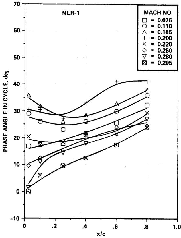
Figure 18.- Phase angle,  $\omega t$ , of flow reversal on NLR-1 airfoil vs chord location for a range of Mach numbers at  $k = 0.1$ ,  $\alpha = 15^\circ + 10^\circ \sin \omega t$  - Mach number effects.
