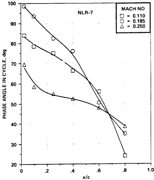
Figure 19.- Phase angle,  $\omega t$ , of flow reversal on NLR-7 airfoil vs chord location for a range of Mach numbers at  $k = 0.1$ ,  $\alpha = 15^\circ + 10^\circ \sin \omega t$  - Mach number effects.
