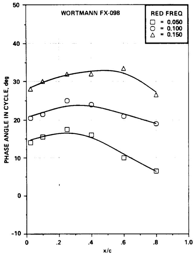
Figure 30.- Phase angle,  $\omega t$ , of flow reversal on Wortmann FX-098 airfoil vs chord for a range of frequencies at  $M_\infty = 0.185$ ,  $\alpha = 15^\circ + 10^\circ \sin \omega t$  - deep-stall conditions.
