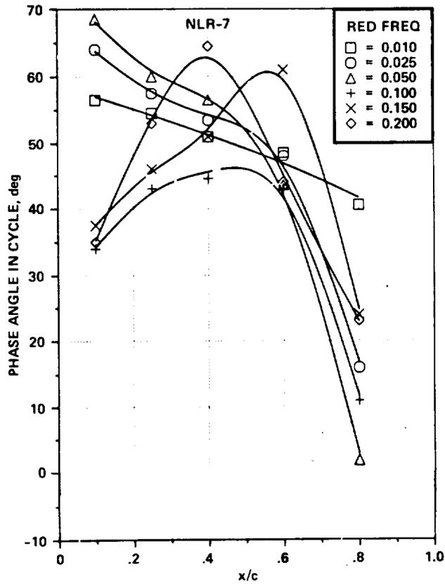
Figure 27.- Phase angle,  $\omega t$ , of flow reversal on NLR-7 airfoil vs chord location for a range of frequencies at  $M_\infty = 0.295$ ,  $\alpha = 15^\circ + 5^\circ \sin \omega t$  - light-stall conditions.
