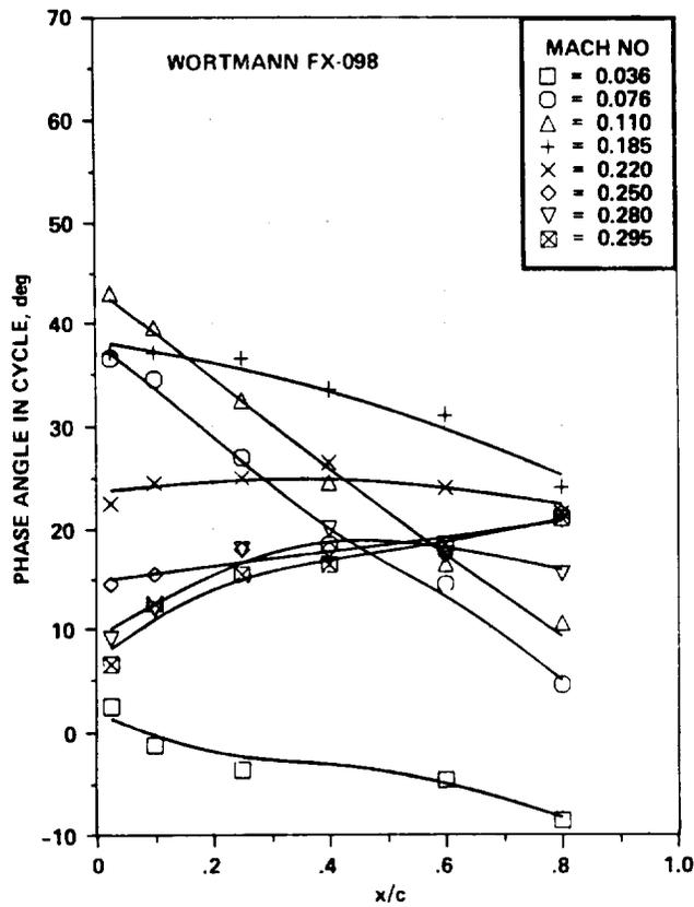
Figure 14.- Phase angle,  $\omega t$ , of flow reversal on Wortmann FX-098 airfoil vs chord location for a range of Mach numbers at  $k = 0.1$ ,  $\alpha = 15^\circ + 10^\circ \sin \omega t$  - Mach number effects.
