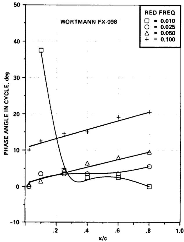
Figure 29.- Phase angle,  $\omega t$ , of flow reversal on Wortmann W-98 airfoil vs chord for a range of frequencies at  $M_\infty = 0.295$ ,  $\alpha = 15^\circ + 10^\circ \sin \omega t$  - deep-stall conditions.
