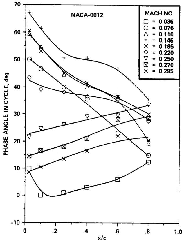
Figure 12.- Phase angle,  $\omega t$ , of flow reversal on NACA 0012 airfoil vs chord location for a range of Mach numbers at  $k = 0.1$ ,  $\alpha = 15^\circ + 10^\circ \sin \omega t$  - Mach number effects.
