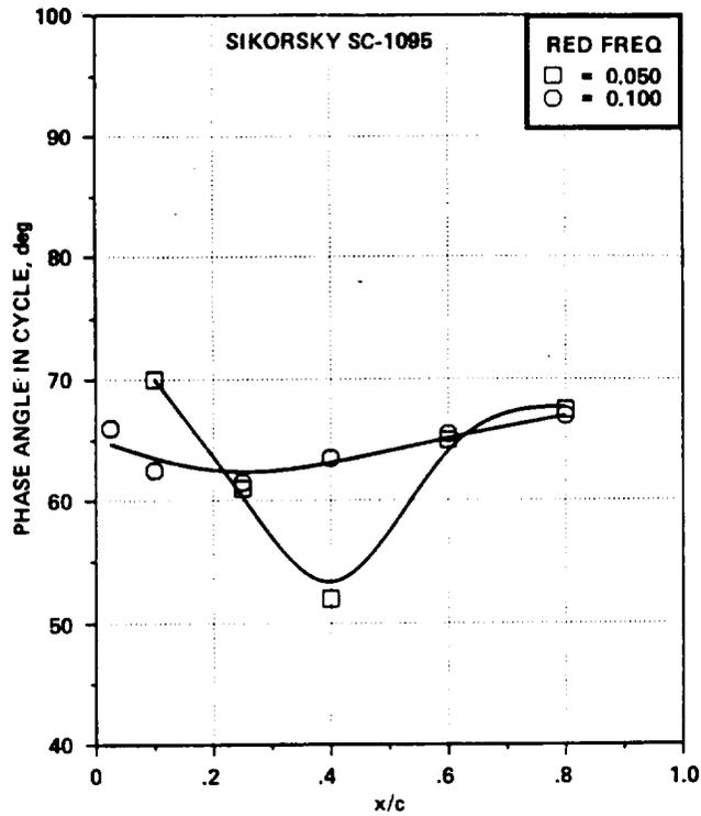
Figure 23.- Phase angle,  $\omega t$ , of flow reversal on Sikorsky SC-1095 airfoil vs chord location for a range of frequencies at  $M_\infty = 0.295$ ,  $\alpha = 11^\circ + 5^\circ \sin \omega t$  - light-stall conditions.
