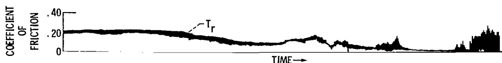
Figure 2. - Typical friction trace for CVM M-50 pin slid on CVM M-50 disk. Temperature range, 218° to 400° C. (See fig. 3(b) for friction-temperature curve.)
