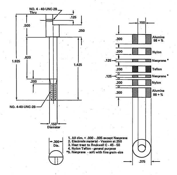
Figure 1. IHPV furnace electrode and pressure seal. Neither the pressure vessel head nor the brass extensions are shown. Base extension attaches to the nipple at the bottom of the electrode; the rod and the cone portion of the electrode are insulated with shrink sleeving. Dimensions are shown as + 0.000, - 0.005 except neoprene which is simply cut to fit.
