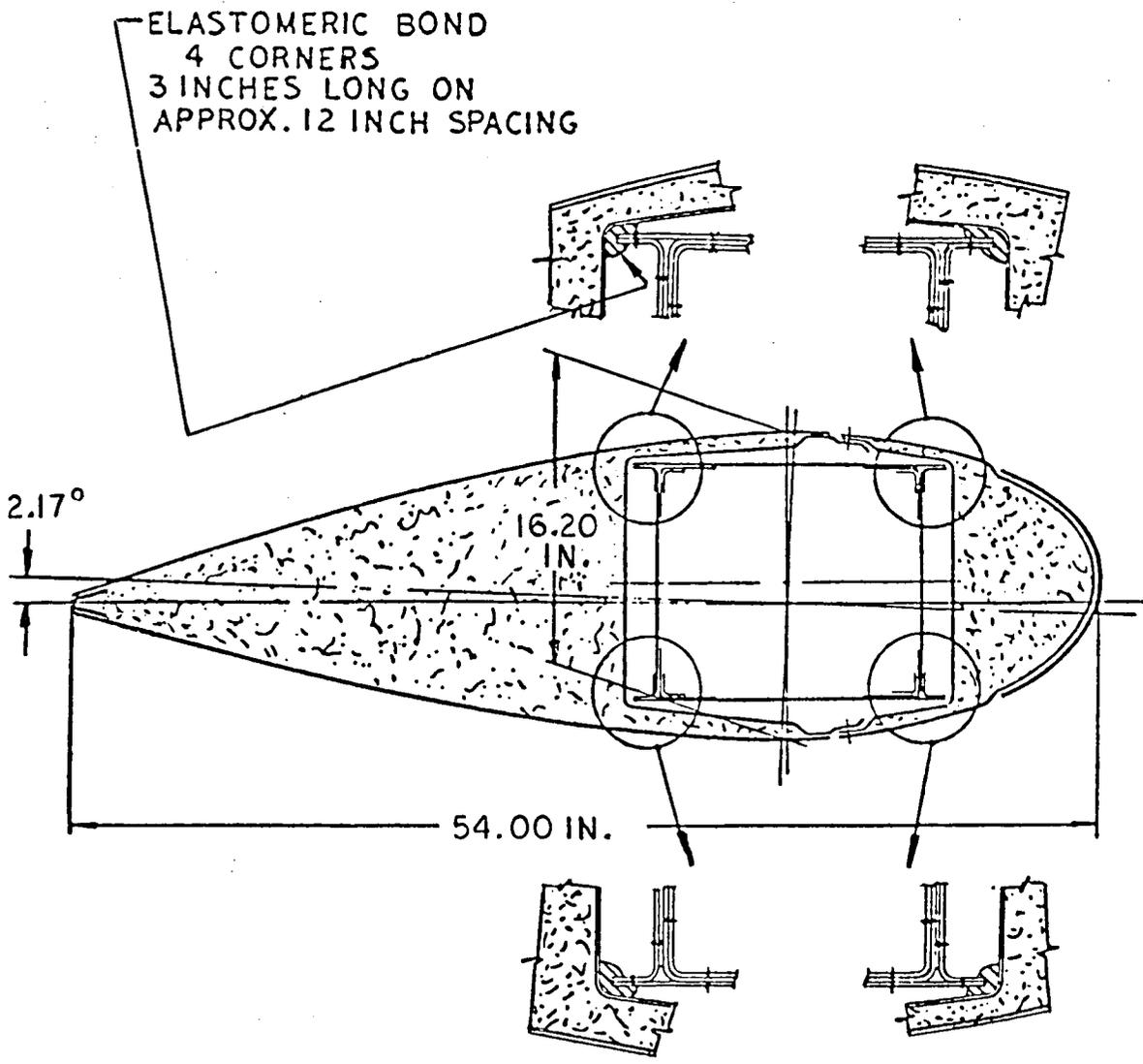
FIGURE 31 - SECTION THRU BLADE - OUTBOARD OF STATION
