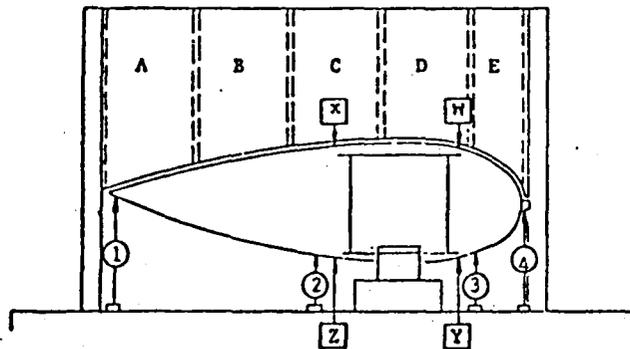
FIGURE 20 - STATIC LOAD TEST (CONFIGURATION)
