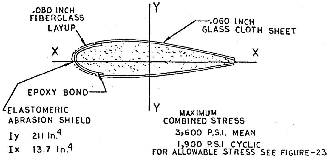
FIGURE 28 - SECTION FIBERGLASS OF TIP EXTENSION
