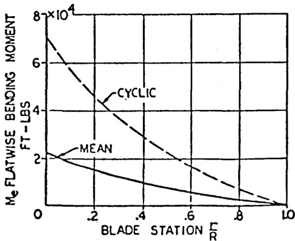
FIGURE 3 - FLATWISE & EDGEWISE BENDING MOMENT DISTRIBUTIONS
