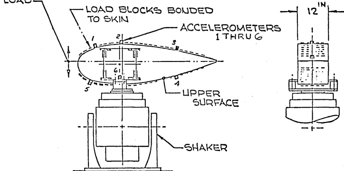
FIGURE 19 - AERODYNAMIC LOADING OF BONDING SURFACES
