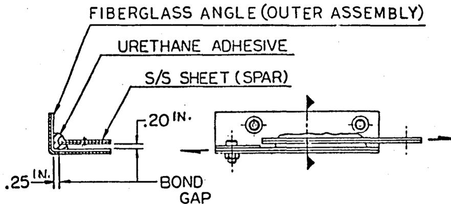
BOND TO STAINLESS STEEL ~1,340 LB./SQ. IN. (NO FAILURE)
