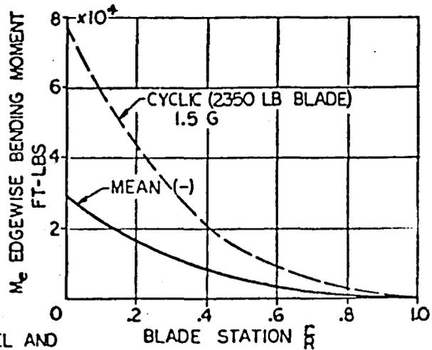
NOTE: THE MOMENT VECTORS ARE PARALLEL AND PERPENDICULAR TO THE .75 CHORD LINE
