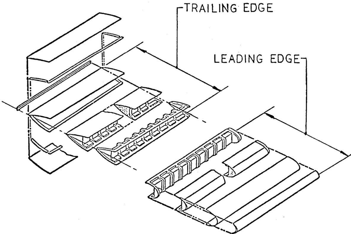
FIGURE 10 - EXPLODED VIEW OF LEADING AND TRAILING EDGE ASSEMBLIES
