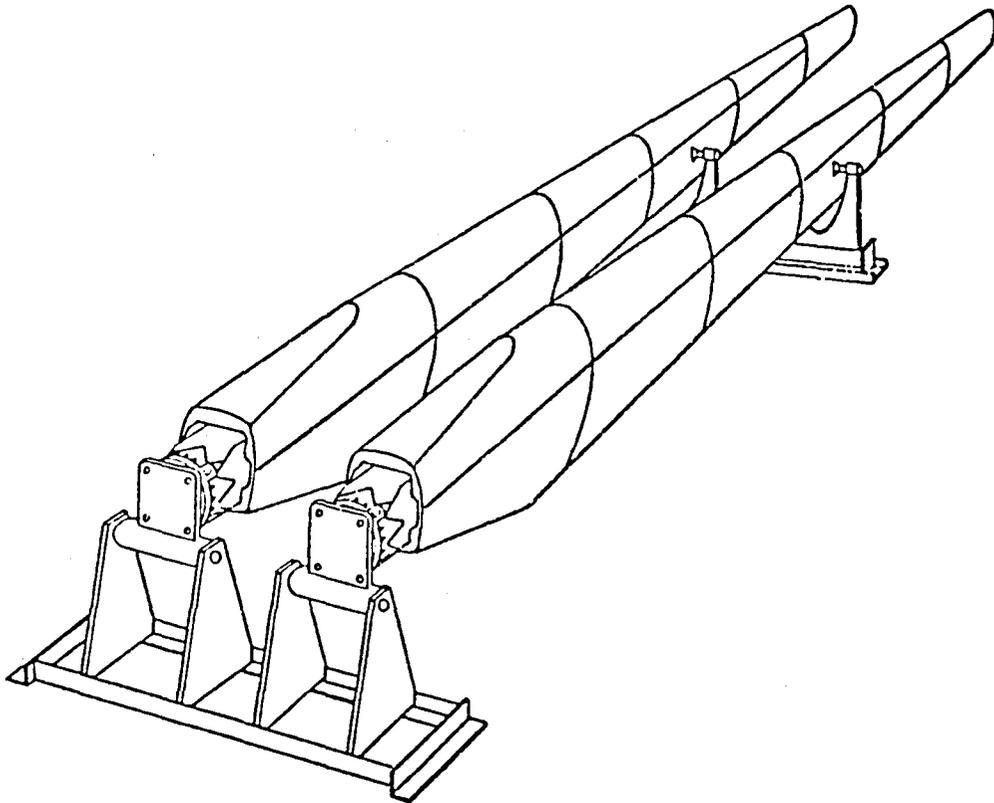
FIGURE 33 - SHIPPING FIXTURE ARRANGEMENT
