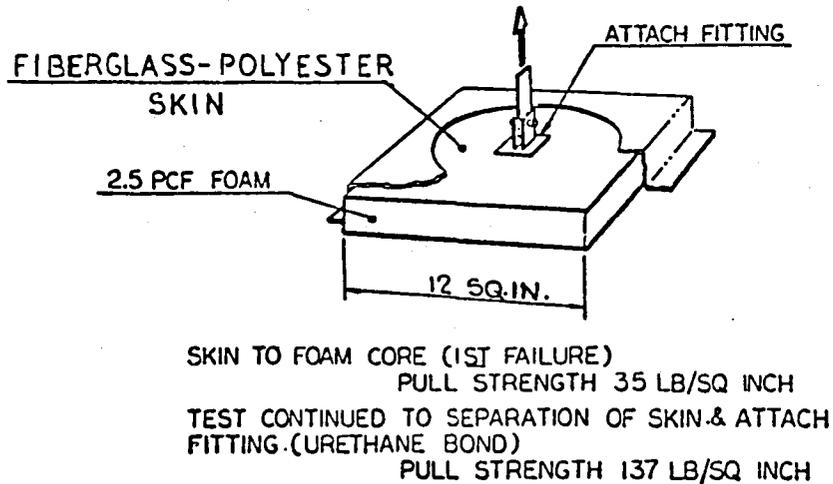
FIGURE 21 - SKIN TO FOAM PULL STRENGTH TEST
