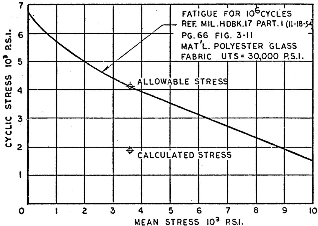
FIGURE 23 - FATIGUE FOR  $10^6$  CYCLES (POLYESTER GLASS)
