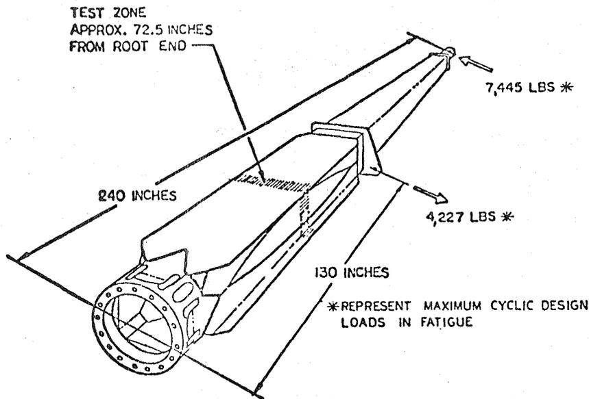
FIGURE 36 - ROOT END TEST BEAM
