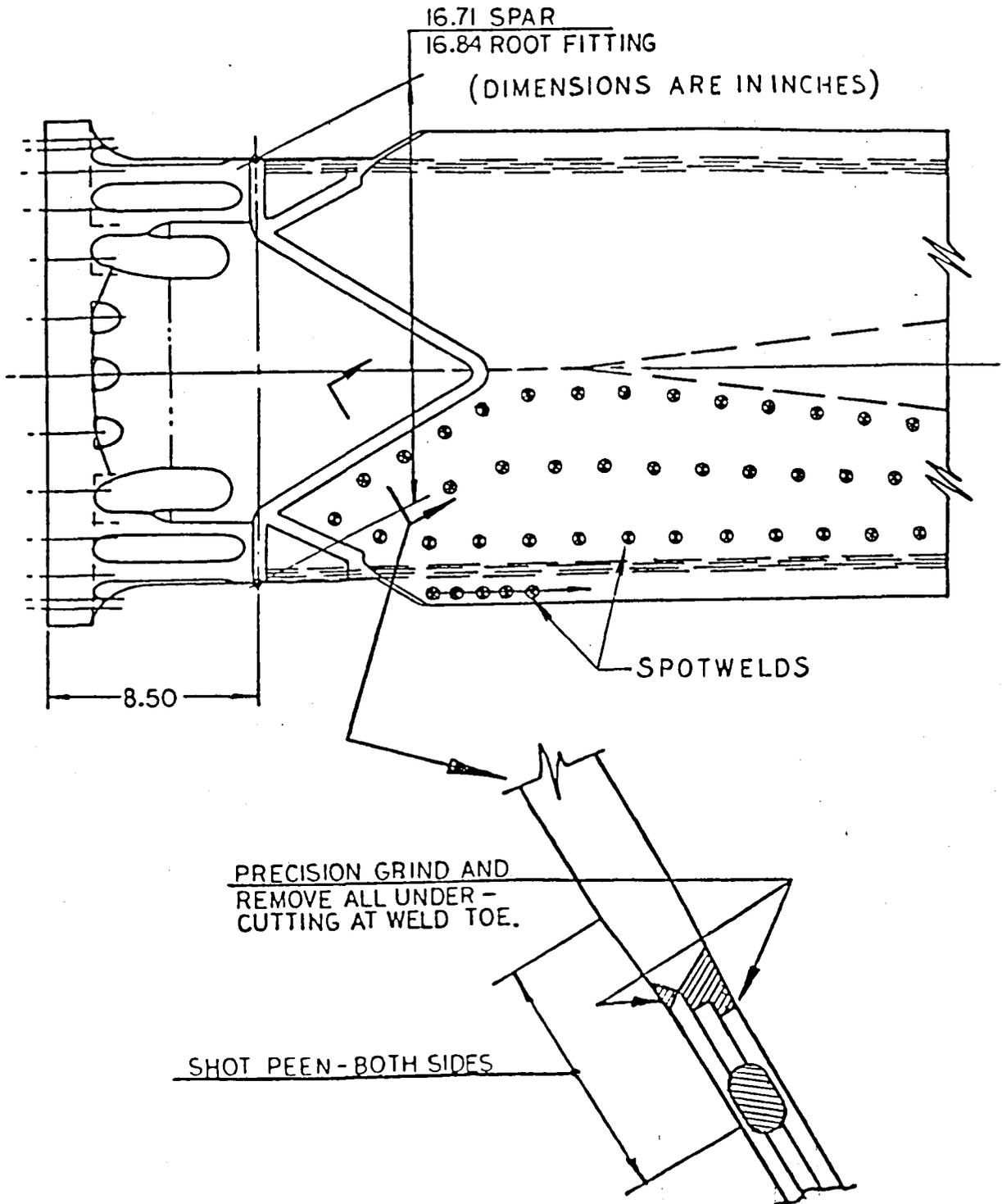
FIGURE 30 - ROOT END - SPAR CONFIGURATION
