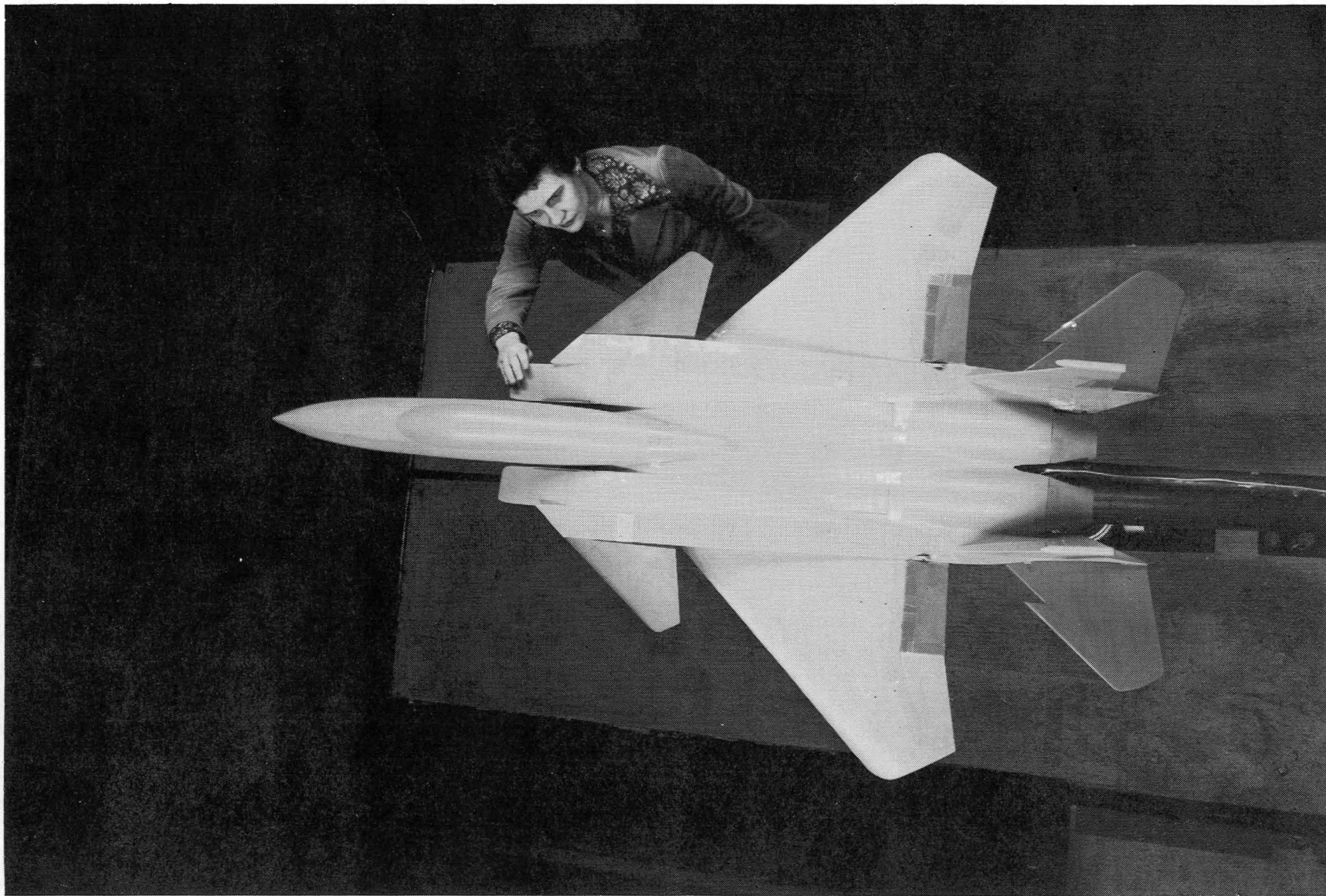
Figure 3.- Photograph of model mounted for static-force tests.
