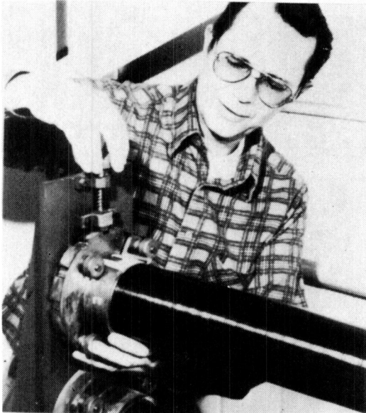
(c) Rotating half-strut for length adjustment.
