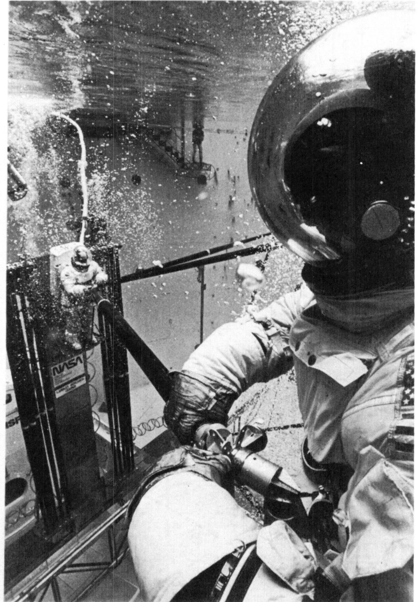
Figure 16.- Installation of strut by two test subjects.
