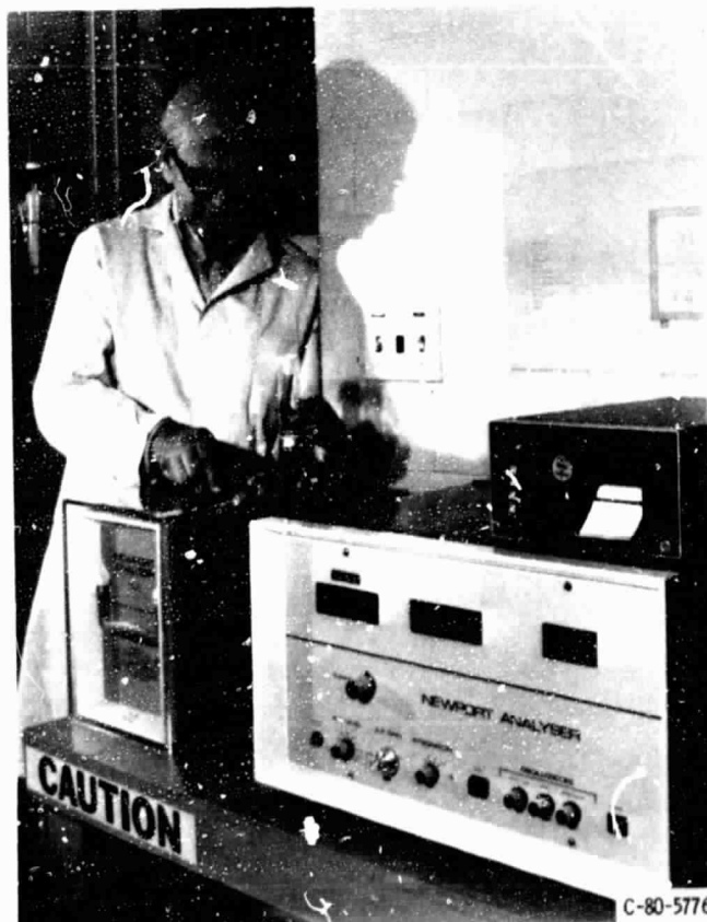
Figure 4. - Nuclear magnetic resonance spectrometer for hydrogen analysis.
