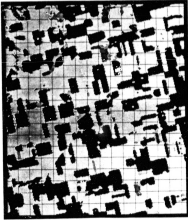
H. FIVE CATEGORY CLASSIFICATION BASED ON TMS BANDS 2, 3, 4 AND 2, 3, 5. AUGUST 30, 1979; WEBSTER, IOWA.
