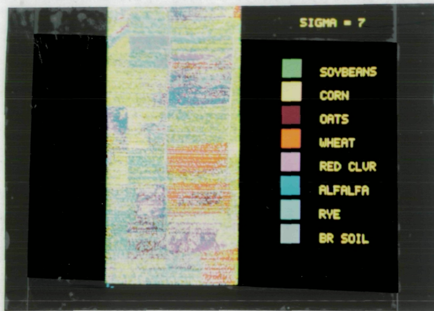
Figure 3.15 Classification results of the original data plus white additive gaussian noise, N(0,7) .
