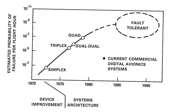
Figure III-3. Digital flight control systems reliability progress.
