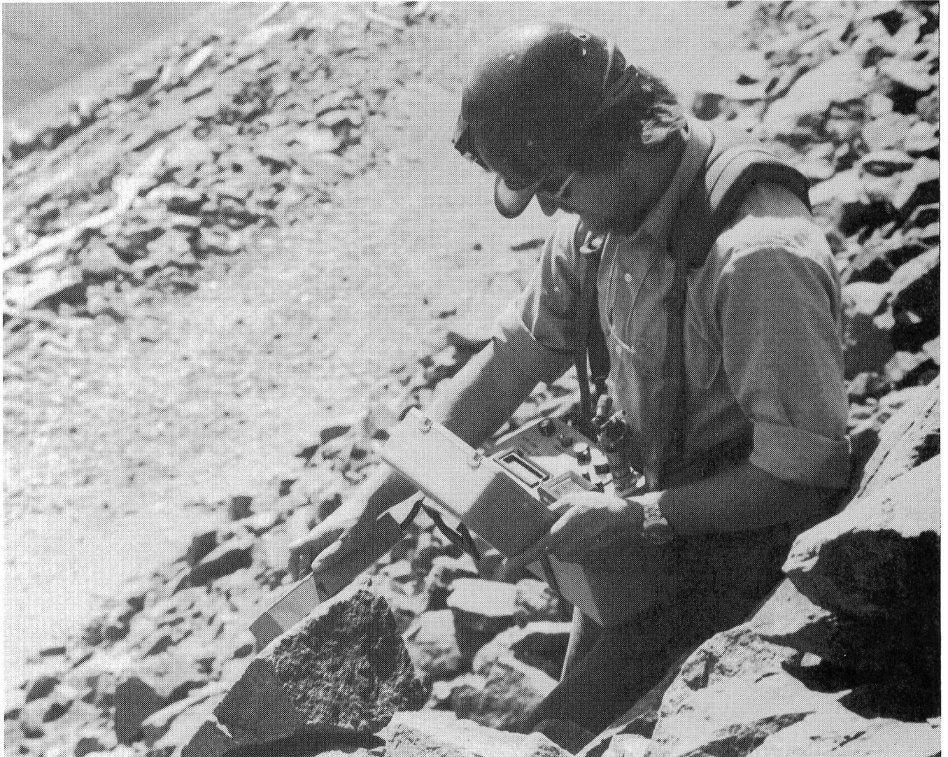
FIGURE 3. - PXRFS as used in the field.
