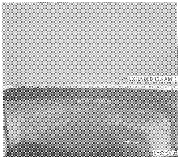
Figure 3. - Photograph illustrating the inelastic extension of ZrO_2-Y_2O_3 beyond the length of the metallic substrate.
