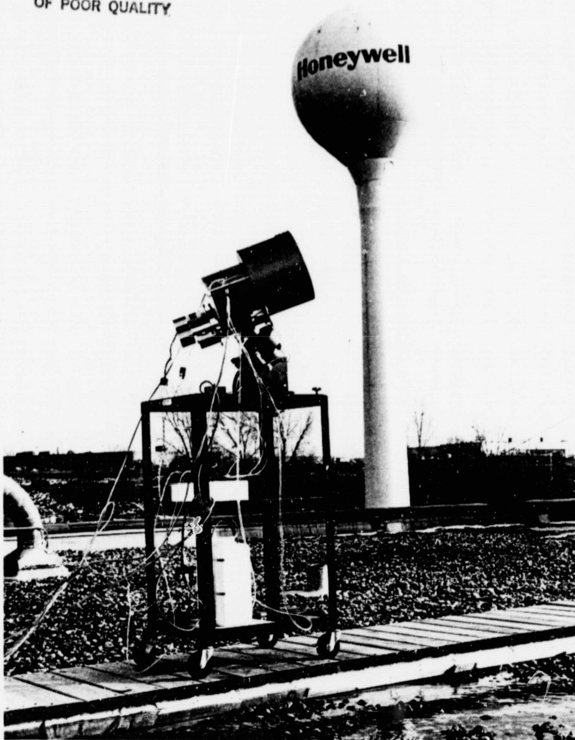
Figure 29. SPV System Test Configuration
