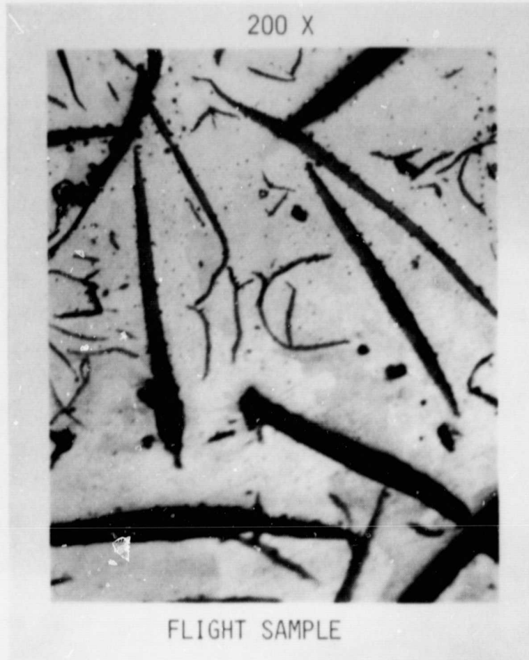
Figure 11. Microstructure for the flight sample 2.5 mm from the primary melt interface.
