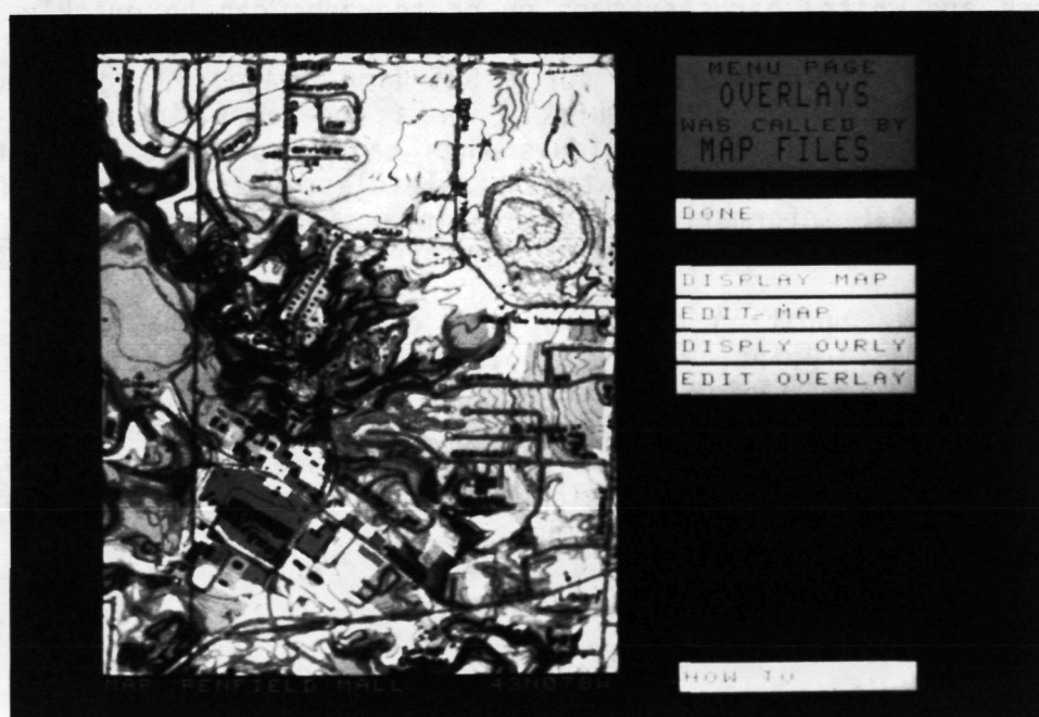
Fig. 2. Color-coded land use information, derived from polygonal data, are registered and displayed over the 1 channel video base map.
