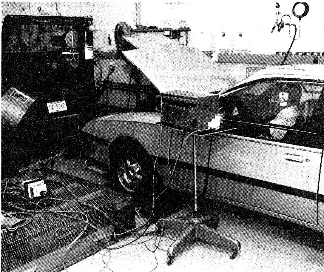
Figure 2-4. ETV-1 Mounted on Clayton Twin-Roll Dynamometer in JPL Automotive Research Facility
