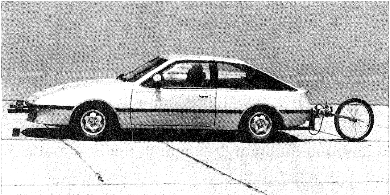
Figure 2-1. ETV-1 During Coastdown Testing at Edwards Air Force Base
