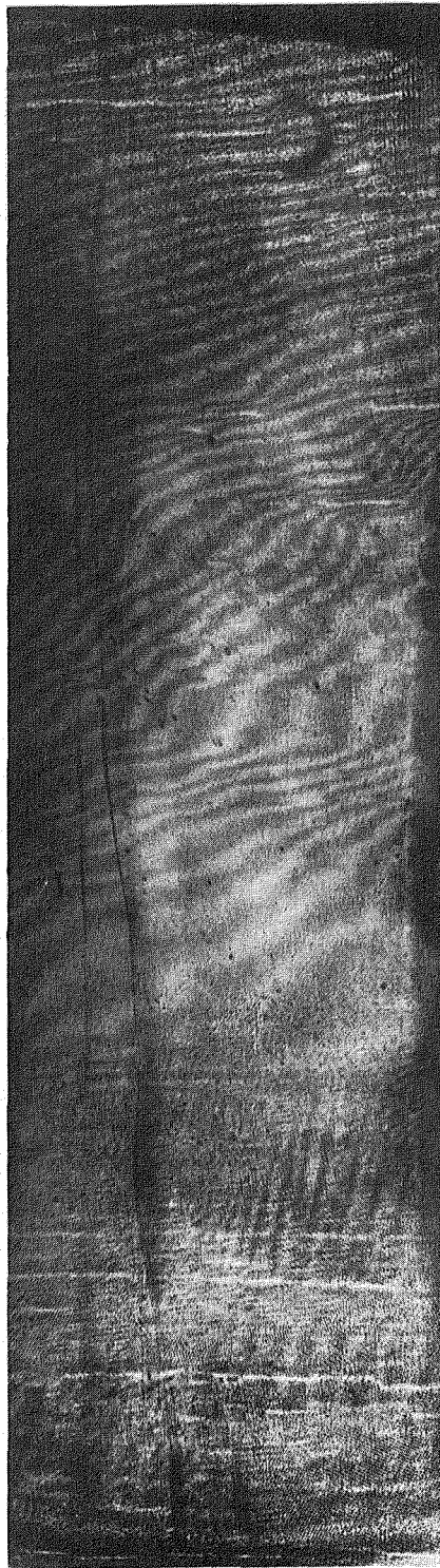
Figure 22. Moiré interferometric pattern obtained when 2000 \mu strain was applied to E-glass epoxy [0,90_3]_S laminate.
