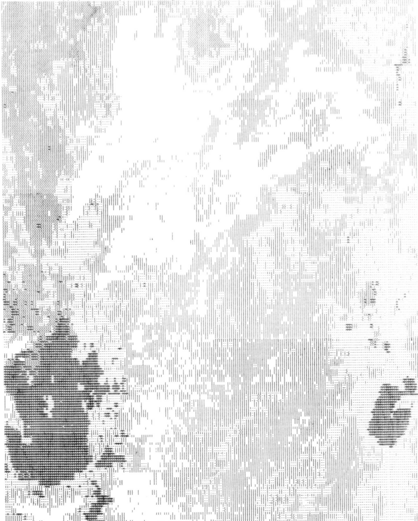
Fig. 12. Example of a symbol coded printout covering the main part of the El Hamma test area. The El Hamma oasis is visible in the lower left corner. The printout is generated after a maximum-likelihood classification of Landsat-1 digital data recorded on Nov. 9, 1972. Each symbol represents one pixel. Aprox. scales: Horizontal 1:60 000 and Vertical 1:70 000. Classes: M=Oasis and irrigated land, -=Cultivated land, I=Grazed steppe, C=Chott, Blank=Overgrazed steppe and desert patch. (Scene 206/36).
