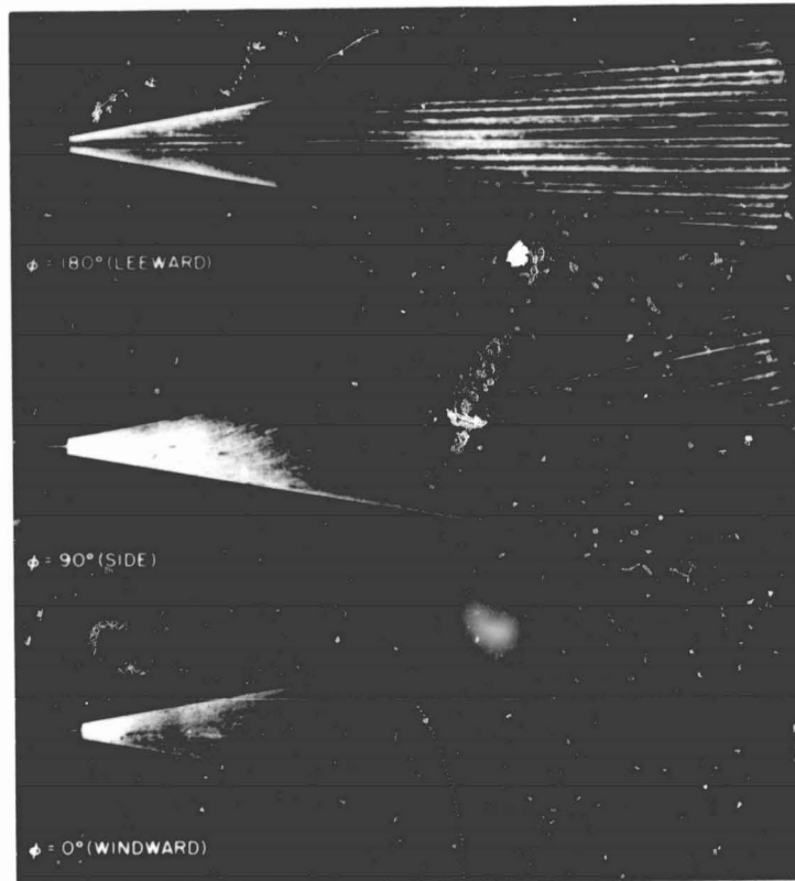
OIL-FILM STUDY ON A 10^\circ SEMI-ANGLE CONE AT \alpha = 5^\circ , M_\infty = 7.4 , R_{L_\infty} = 3 \times 10^6 , T_T = 1050^\circ\text{K} , (McDEVITT AND MELLENTIN 1969)
