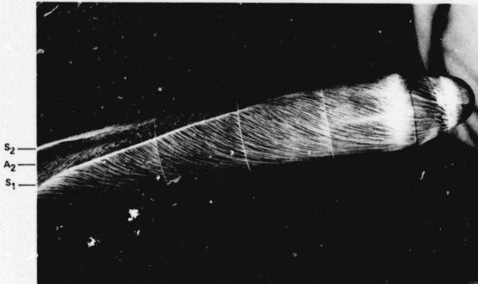
(a) SIDE ELEVATION, R_{L_{\infty}} \sim 10 \times 10^6 , R_D = 1.3 \times 10^6 LENGTH, L = 38.2 cm (15 in.); D = 5.0 cm (1.97 in.)
