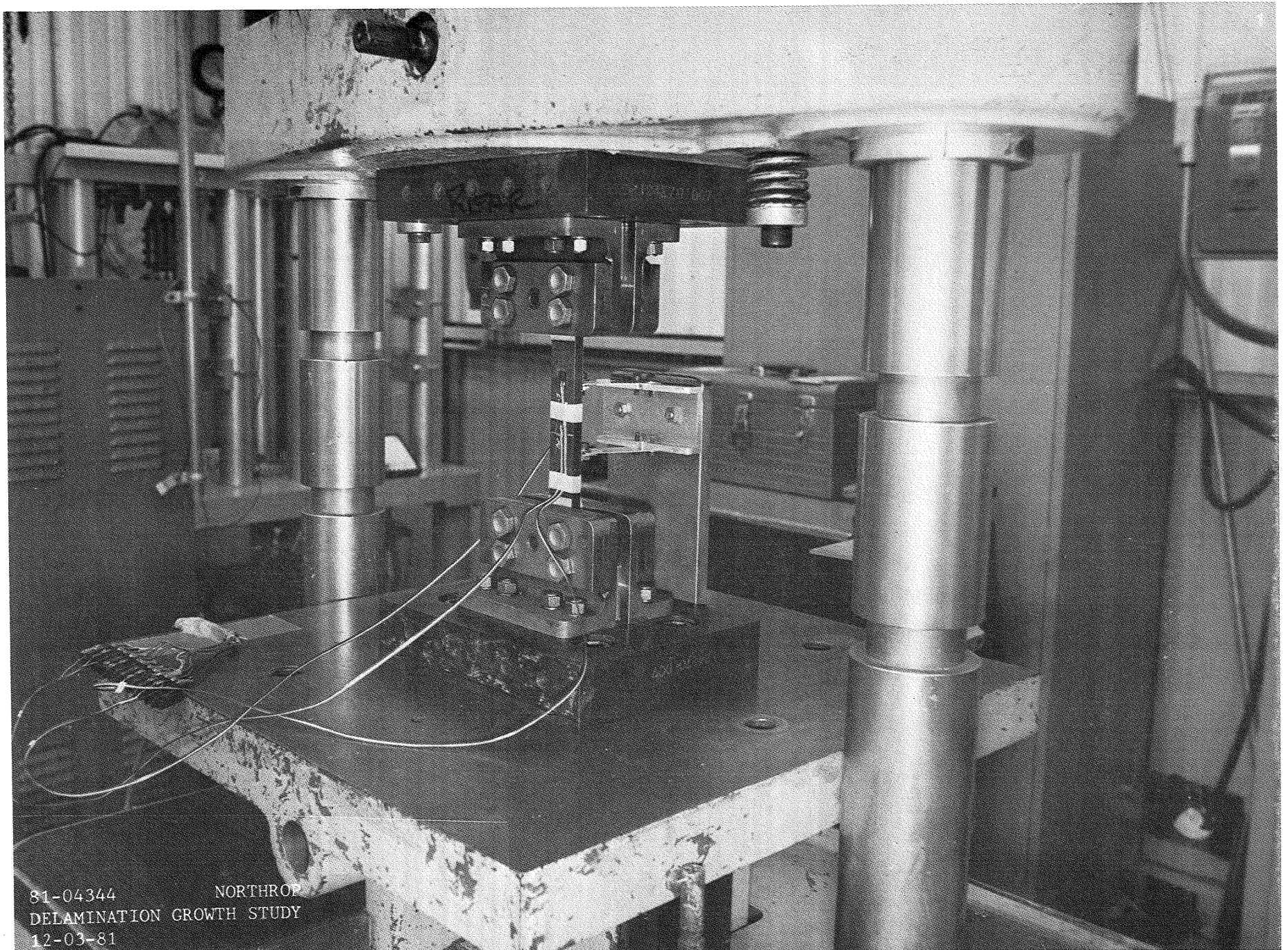
Figure 9. Static Compression Test Setup for Specimens With ITTW Delaminations.
