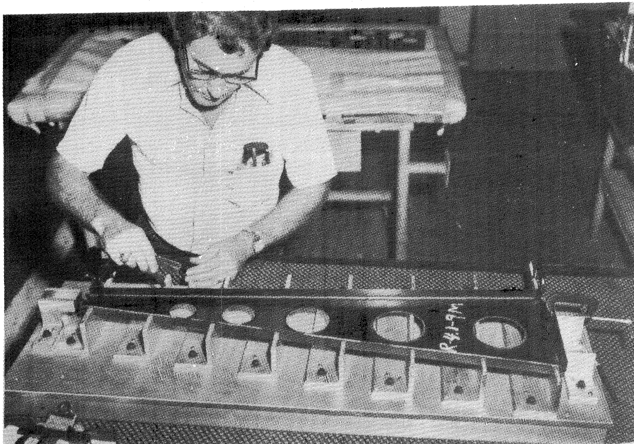
Figure 56. - Rib dimensional check fixture.
