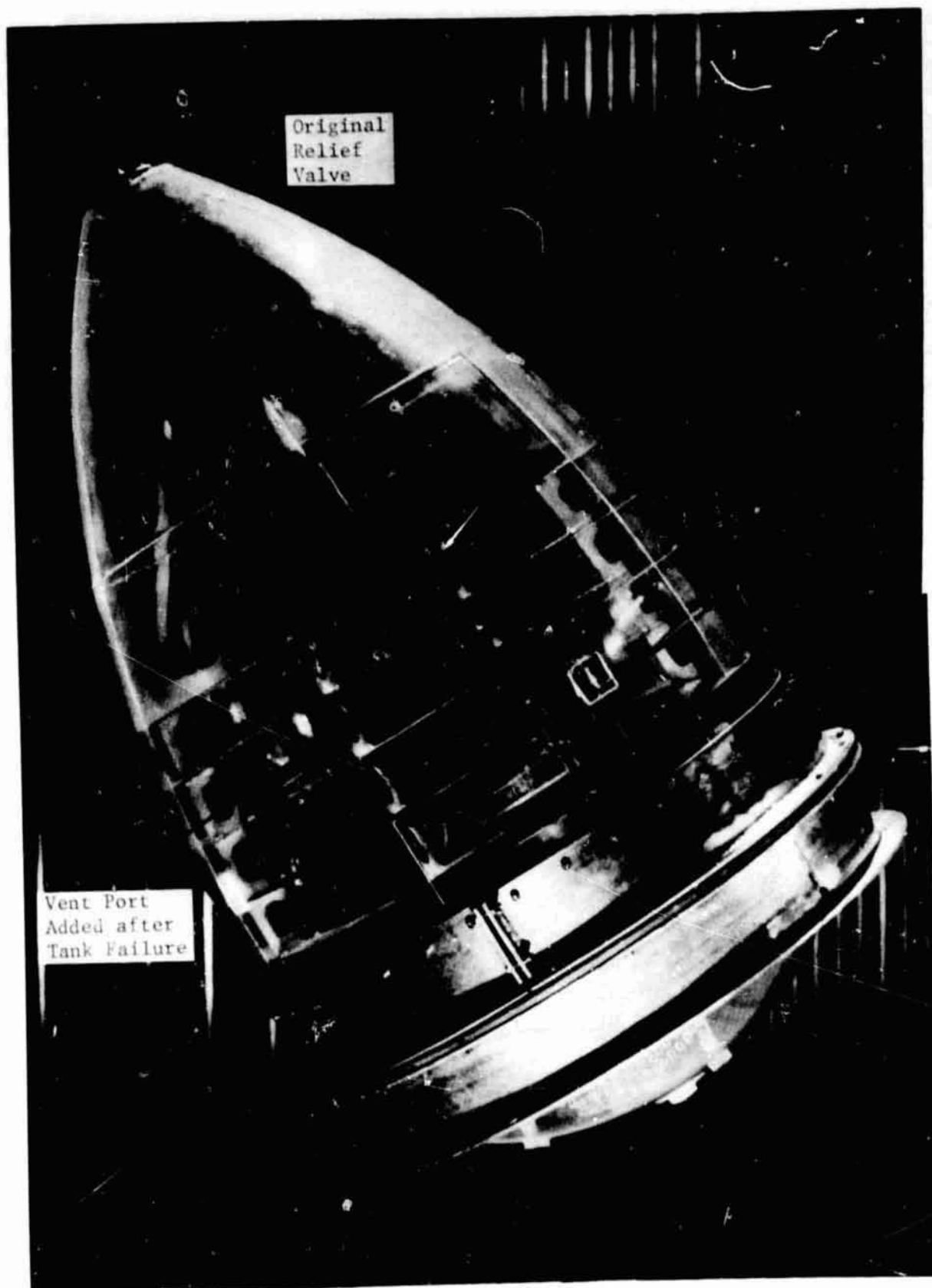
Figure 2-16. Repaired 1/10th-Scale Tank
