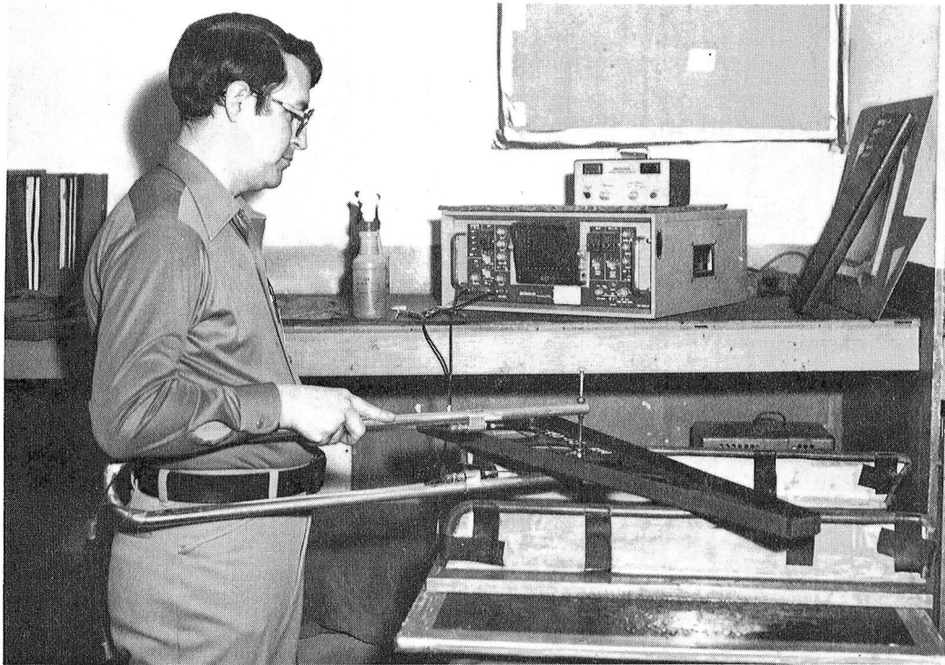
Figure 19. - Ultrasonic Inspection of Cured Rib Detail
