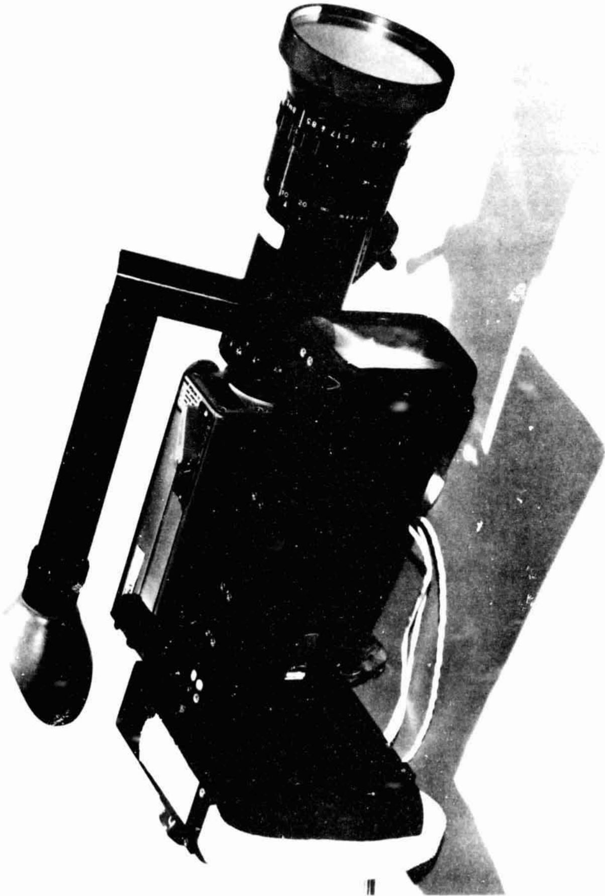
Figure 1: Instrumentation package comprising 16 mm motion picture camera and photocell sensor.
