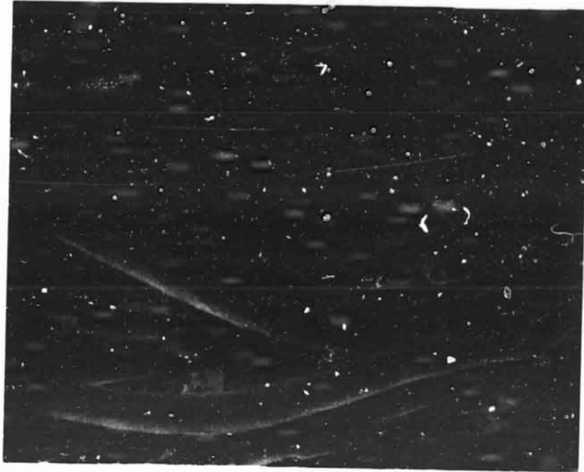
Figure 4. Green fibers from failed vent line.
