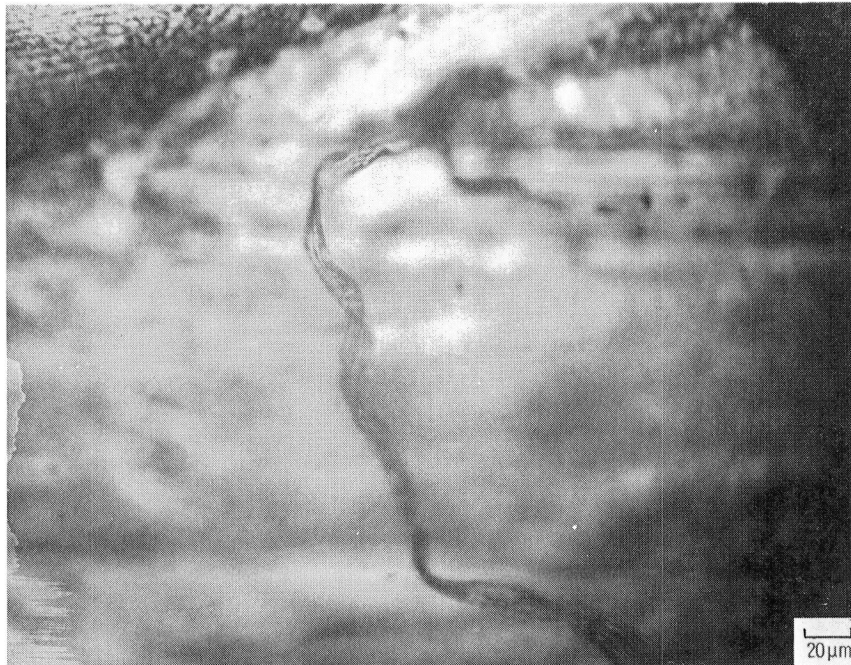
Figure 14. - Fibril type of wear debris (test 1, 42K cycles).
