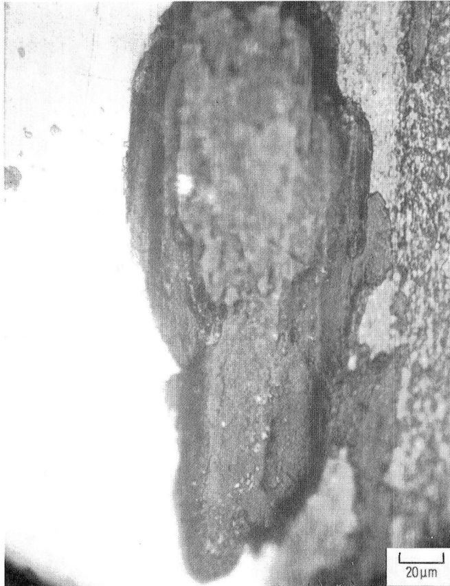
Figure 15. - Dark patch type of wear debris (test 2, 1015K cycles).
