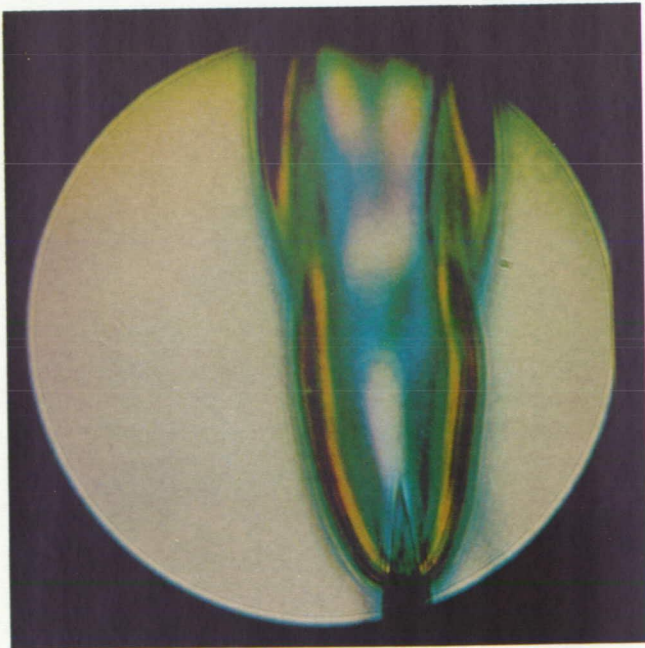
Figure 6. - Rainbow schlieren photograph of acetylene torch operating unstably.
