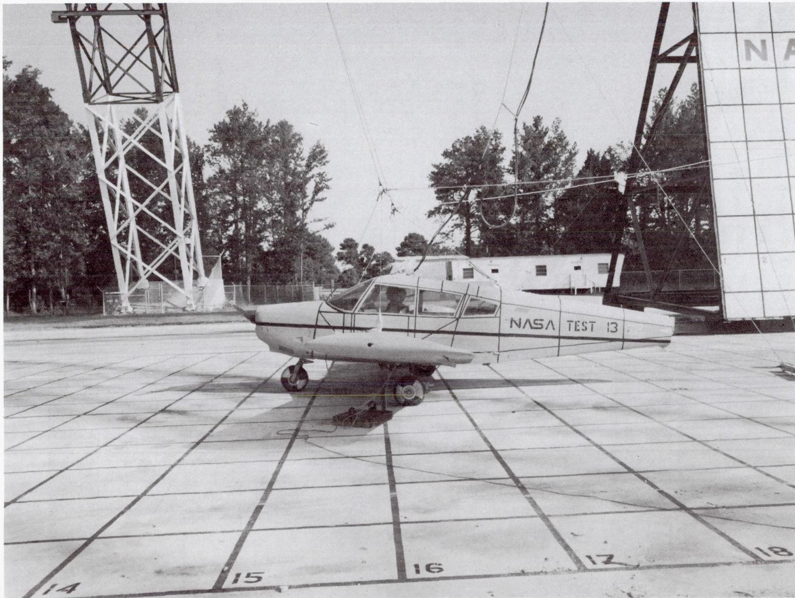
Figure 7.- Typical airplane test specimen in crash-test preparation.
