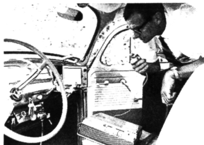
FIGURE 3. The meter of a thermistor thermometer is temporarily mounted on the glove compartment lid with an extension of the vehicle's instrument lighting system in front of the meter for a light. It is advisable to have either a tape recorder or a passenger to record the observations.
