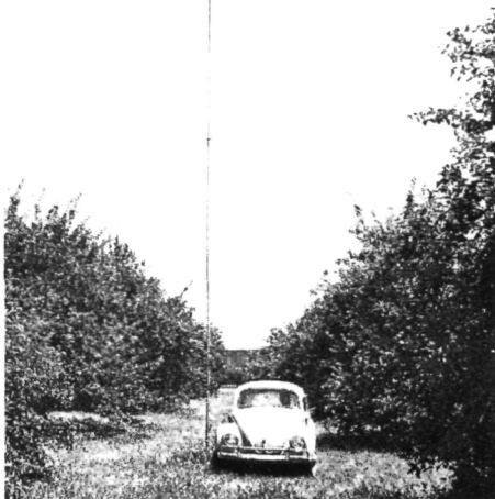
FIGURE 4. A 50 foot tower for monitoring temperature inversion, showing the vehicle at the base of the tower where wires connected to thermistors on the tower are momentarily plugged into a meter in the vehicle to sense air temperatures at various levels on the tower. With practice, the observer can make his notations and drive away from the tower before the effect of the vehicle on temperature readings becomes noticeable.
