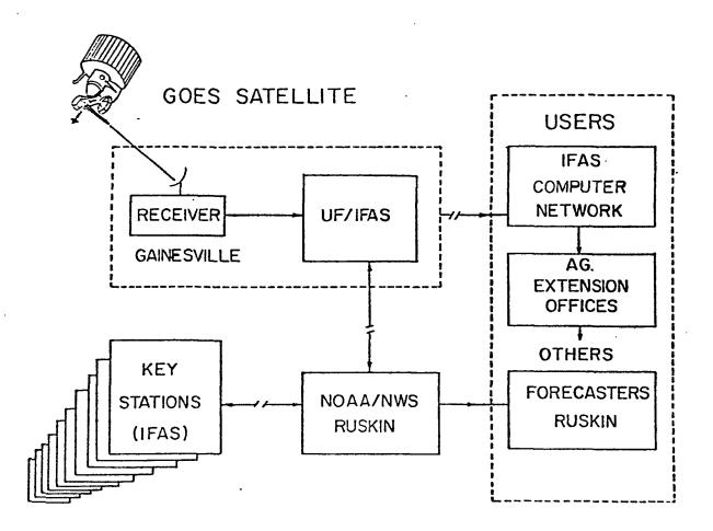
Fig. 7. Block diagram of SFFS when the antenna at UF/Gainesville (Fig. 7) becomes operational. Dissemination of SFFS products is expected to rely heavily on the IFAS computer network that is expected to link the county extension offices with the main campus of UF. Compare with Figure 1.
