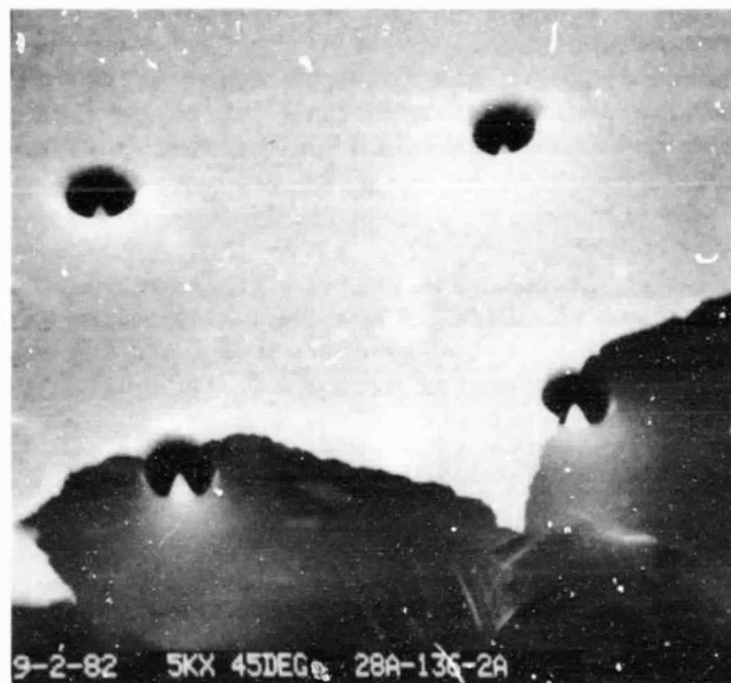
(b) ANISOTROPIC DRY ETCH OF \text{SiO}_2 TIPS ON 9\text{-}\mu\text{m} CENTERS
