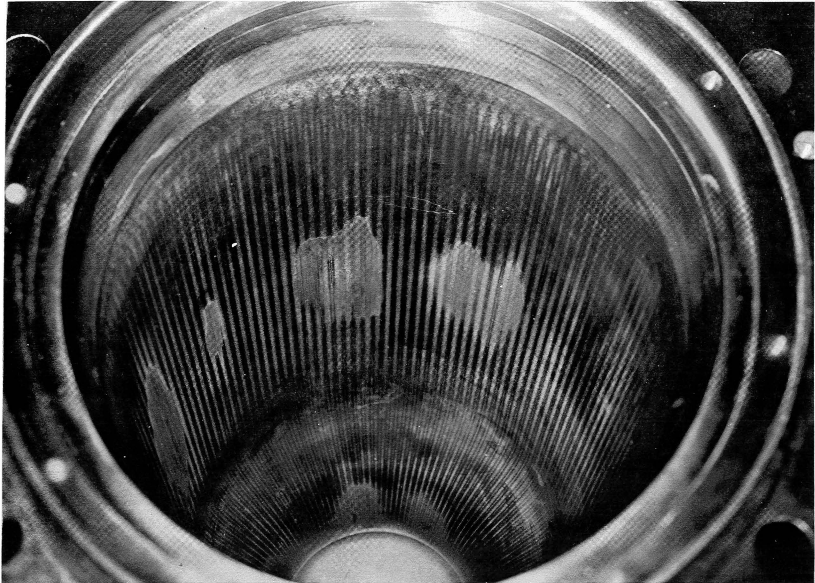
Figure 78. 40K MCC Showing Anomalous Injector Effects
