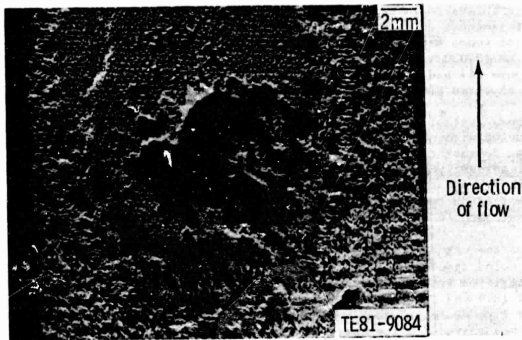
Figure 25. 0.38 mm (0.015 in.) knit--severe erosion, 30 min, 45° angle (X5).
