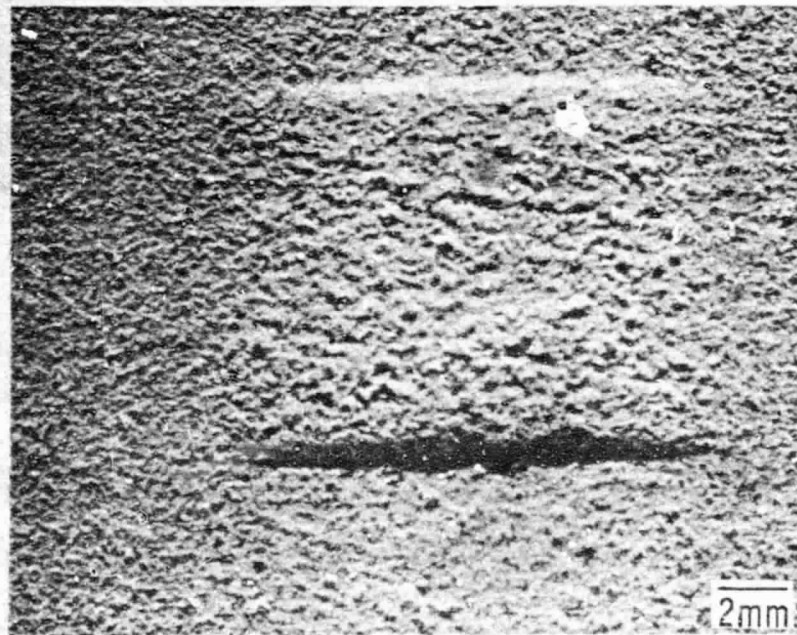
B. 30/70% composition 10000 rpm rub-SiC blade tip 0.40 mm (0.016 in.) deep
