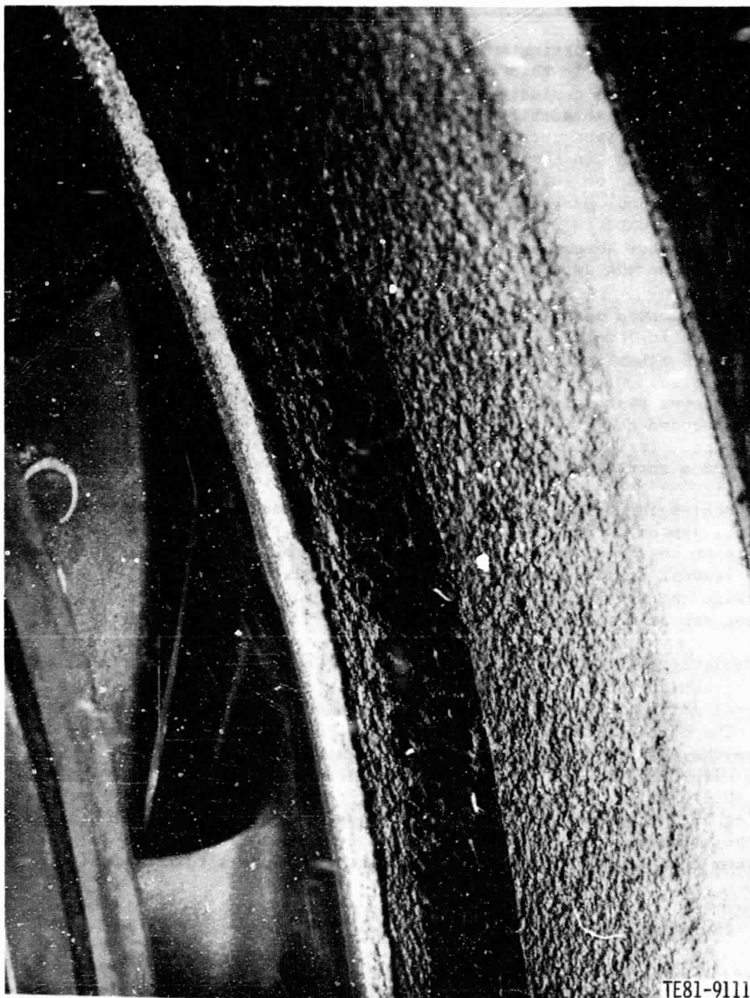
Figure 53. Turbine tip rub on zirconia/eccosphere abrasion-resistant coating. Rotor material is Mar-M246.
