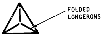
Figure 1.4-12. End View of Folded Configuration
