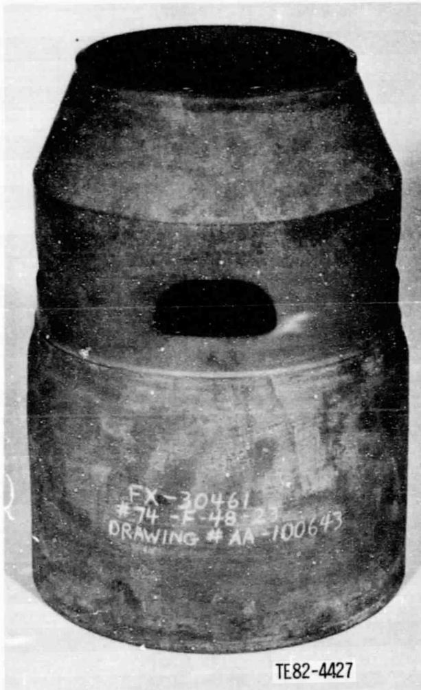
Figure 58. Machined CBO combustor body.
