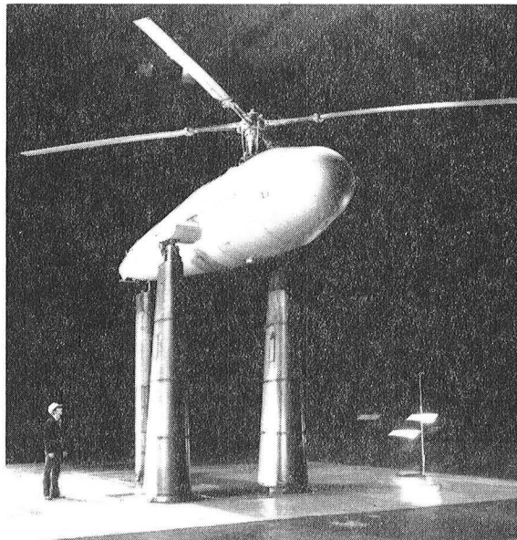
Fig. 2. Full-scale rotor test apparatus in the Ames 40- by 80-Foot Wind Tunnel.
