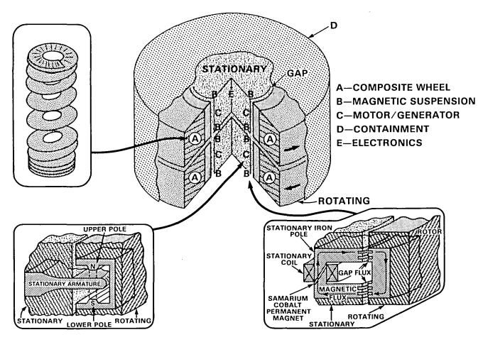
Figure 1.- Spacecraft flywheel power system: conceptual flywheel design.
