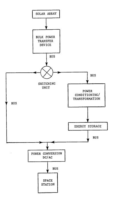
In the chart below, efficiencies have been assigned to each element of the power system. This must be done so that the required array size can be determined, and so that the sensibilities of the system can be examined by changing each item. Also, it should be obvious that the most efficient method of operating the station is to cycle the high loads on during the sun portion of the orbit so that the storage system is not utilized.
