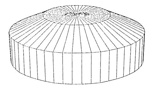
SINGLE WHEEL ENERGY STORAGE ONLY By adding a second counter rotating wheel, it is possible to provide energy storage without disturbing the attitude control system. But since two wheels will provide control of two functions, it is now possible to provide single axis attitude control essentially for free in addition to the energy storage function.
