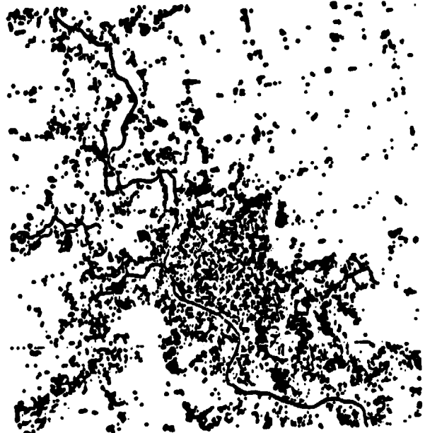
Fig. 10 Results of Linear Feature Detection for Iowa Test Area, Band 5, Dark Lines
