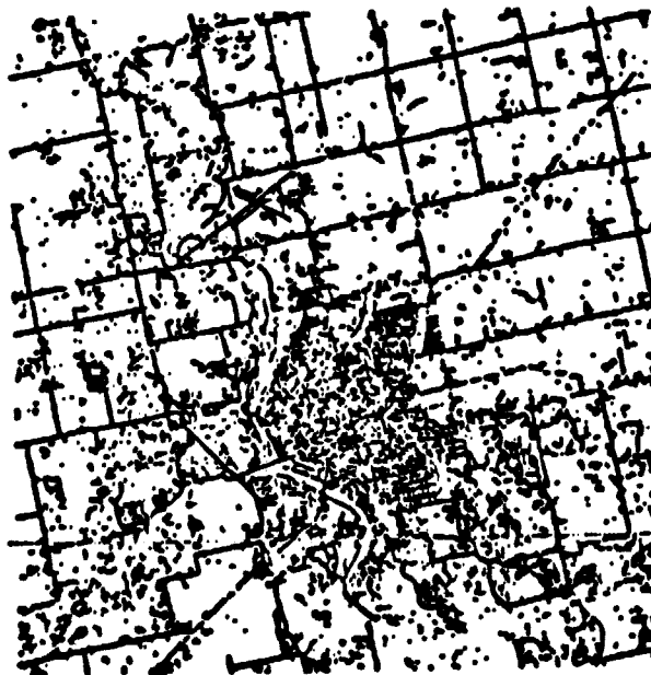
Fig. 8 Results of Linear Feature Detection for Iowa Test Area, Band 7
