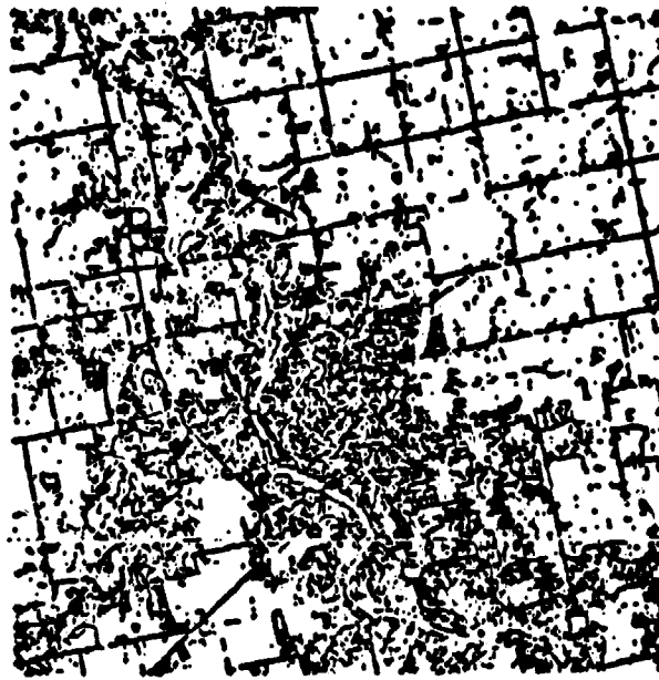
Fig. 7 Results of Linear Feature Detection for Iowa Test Area, Band 5
